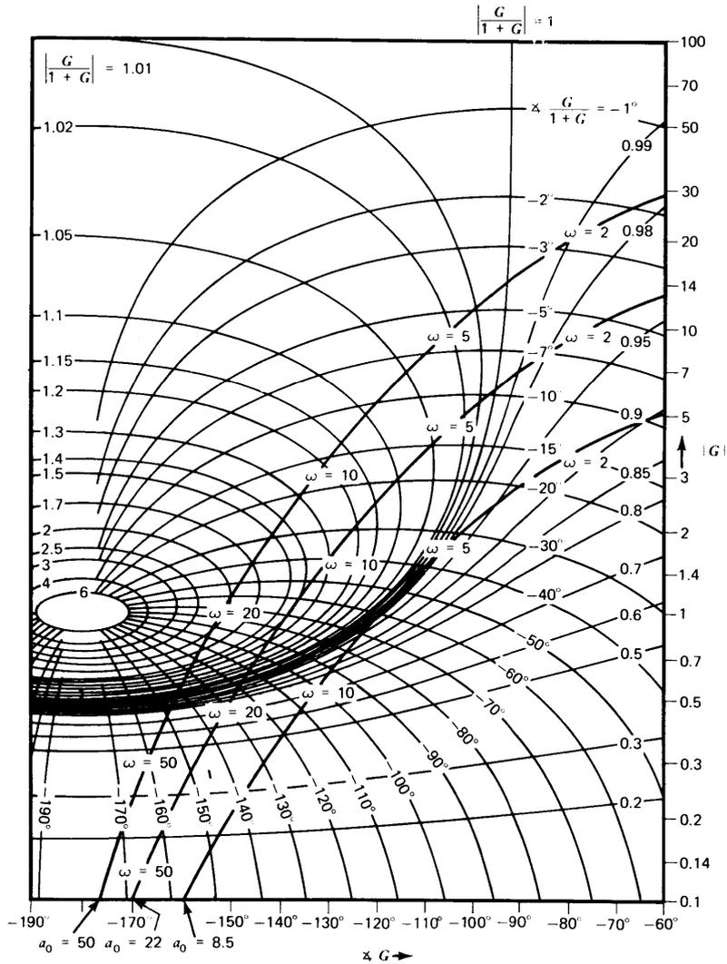
**Determination of closed-loop transfer function for  $a(s) = a_0 / [(s + 1)(0.1s + 1)]$ ,  $f = 1$ .**
