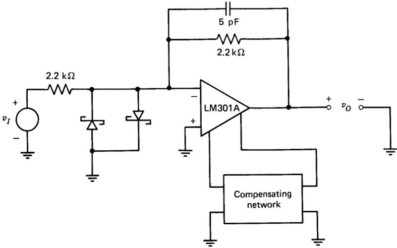
**Figure 13.44** Inverter used to evaluate large-signal response.
