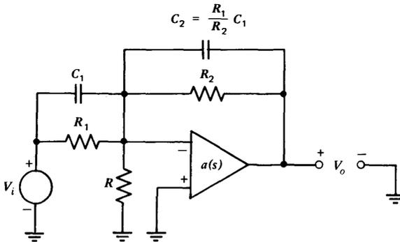
Figure 13.2 Lead compensation for the inverting amplifier connection.
