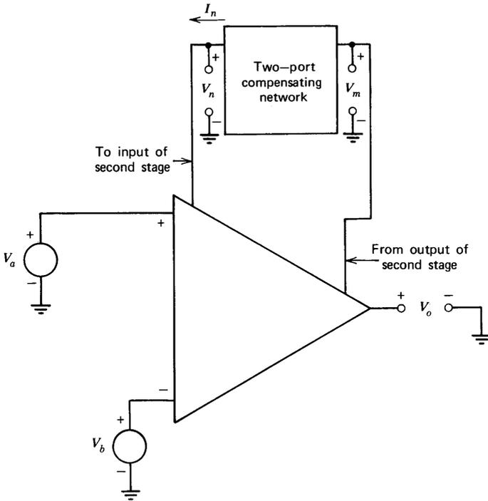
**Figure 13.11** Operational amplifier compensated with a two-port network.
