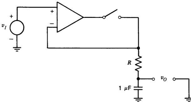
Figure 13.51 Sample-and-hold circuit.
