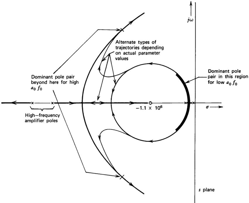
Figure 13.23 Root-locus diagram for inverter with two-pole compensation.
