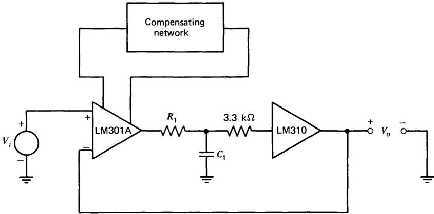
Figure 13.32 Circuit used to evaluate slow-rolloff compensation.
