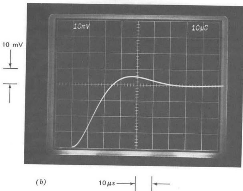
**Figure 13.39** Step response for system with slow-rolloff compensation as a function of  $R_1C_1$ . (Input-step amplitude = 40 mV.) (a)  $R_1C_1 = 10 \mu\text{s}$ . (b)  $R_1C_1 = 100 \mu\text{s}$ . (c)  $R_1C_1 = 1 \text{ ms}$ . (d)  $R_1C_1 = 10 \text{ ms}$ . (e)  $R_1C_1 = 100 \text{ ms}$ .
