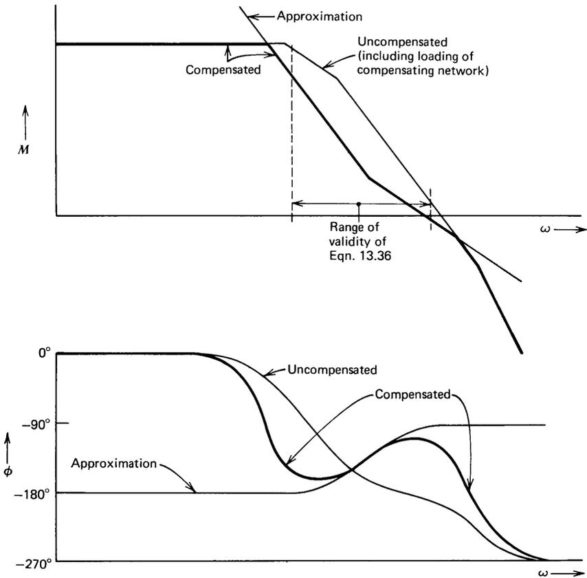
**Figure 13.20** Open-loop transfer function for two-pole compensation.
