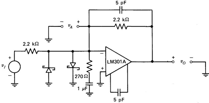
**Figure 13.47** Unity-gain inverter with input lag compensation.
