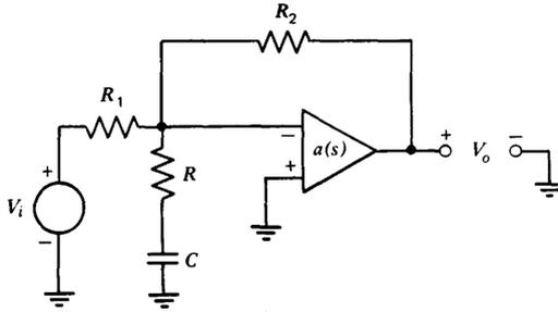
Figure 13.1 Lag compensation for the inverting amplifier connection.
