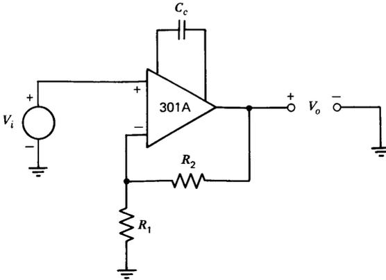
**Figure 13.14** Noninverting amplifier.
