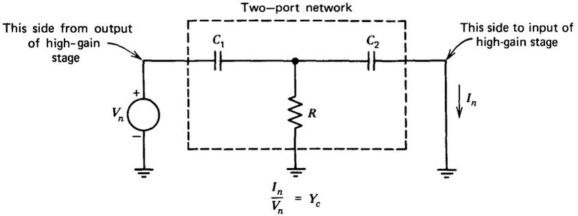
Figure 13.19 Network for two-pole compensation.
