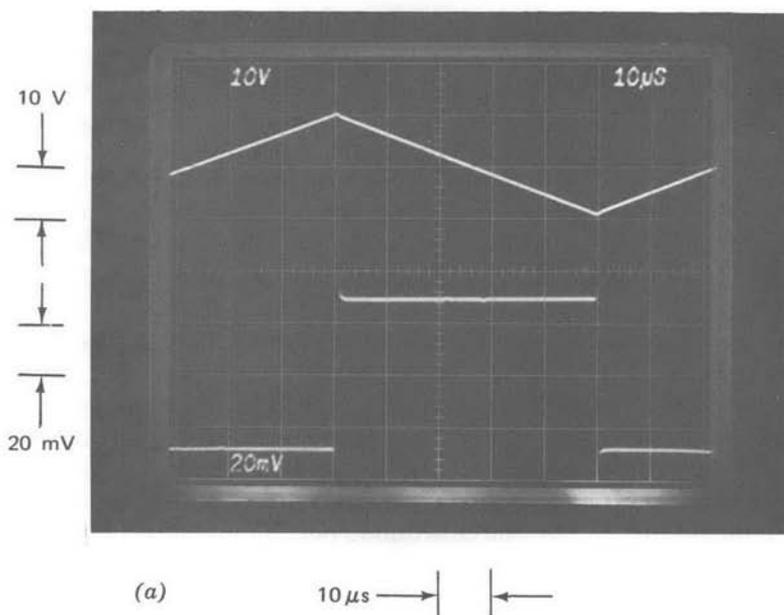
**Figure 13.24** Unity-gain inverting-amplifier response with triangle-wave input. (Input amplitude is 20 volts peak-to-peak.) (a) One-pole compensation—upper trace: output; lower trace: inverting input of operational amplifier. (b) Two-pole compensation—upper trace: output; lower trace: inverting input of operational amplifier. (c) Repeat of lower trace, part b, with faster sweep speed.
