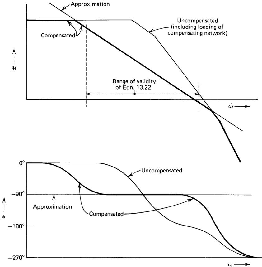
**Figure 13.12** Open-loop transfer function for one-pole compensation.
