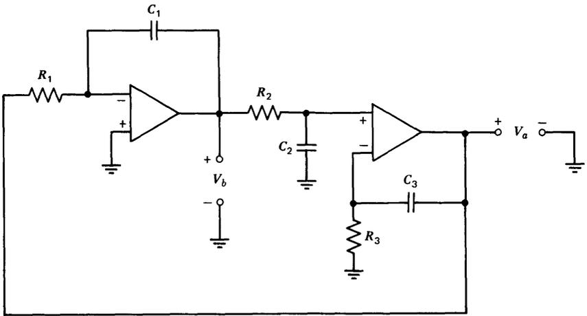
**Figure 12.2** Quadrature oscillator.
