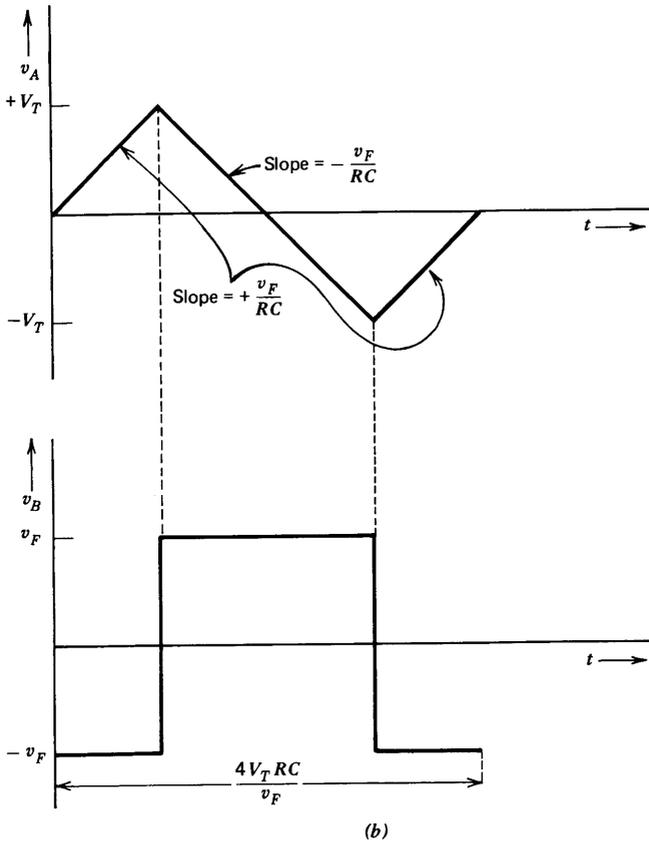
**Figure 12.10** Voltage-controlled oscillator. (a) Circuit. (b) Waveforms.
