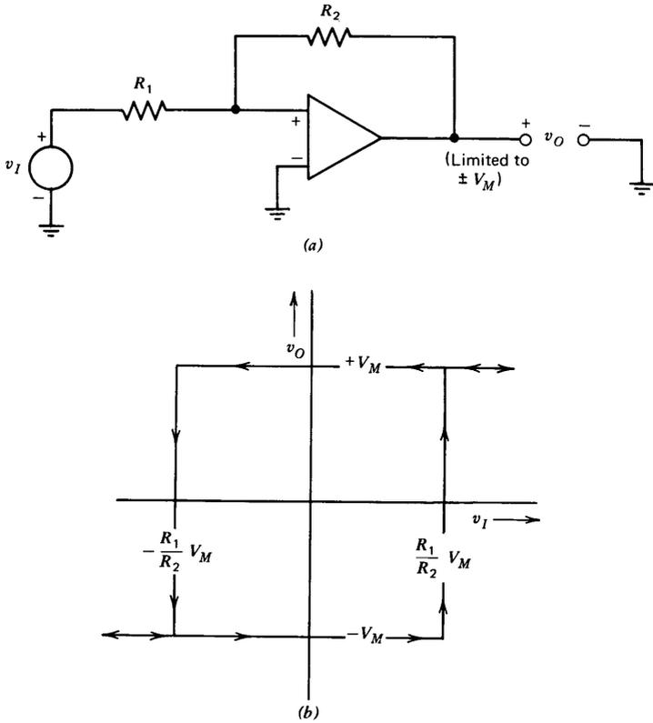
**Figure 12.7** Schmitt trigger. (a) Circuit. (b) Characteristics.
