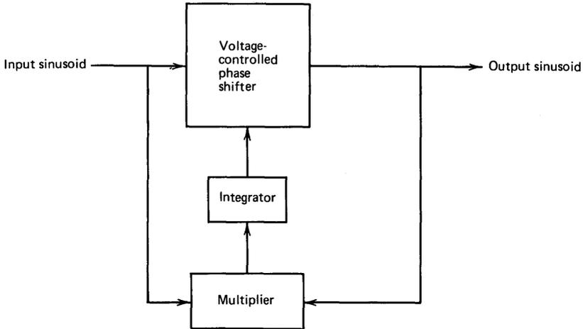
**Figure 12.31** Constant phase shifter using a phase detector.
