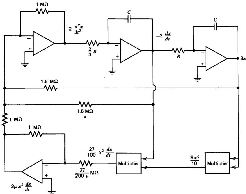
Figure 12.16 Scaled simulation of Van der Pol's equation.
