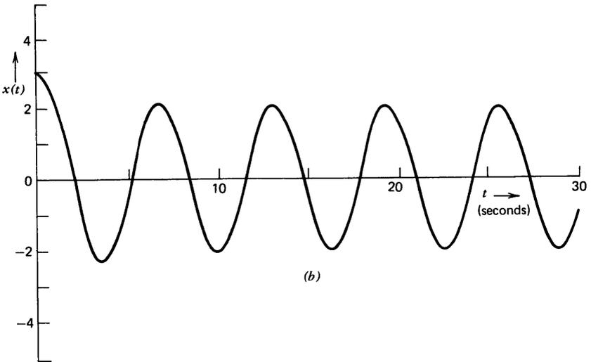
**Figure 12.15** Solution to  $d^2x/dt^2 + 0.25(x^2 - 1)(dx/dt) + x = 0$ . (a) With initial conditions  $x(0) = 0.5$ ,  $(dx/dt)(0) = 0$ . (b) With initial conditions  $x(0) = 3$ ,  $(dx/dt)(0) = 0$ , (c) Parts a and b repeated in phase-plane form.
