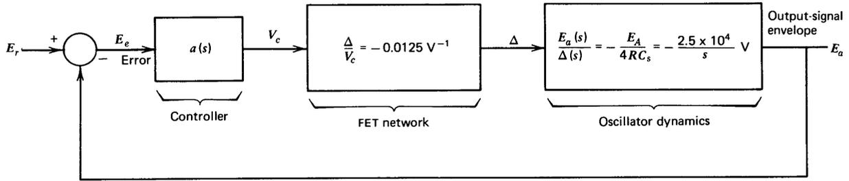
Figure 12.5 Linearized block diagram for amplitude-control loop.
