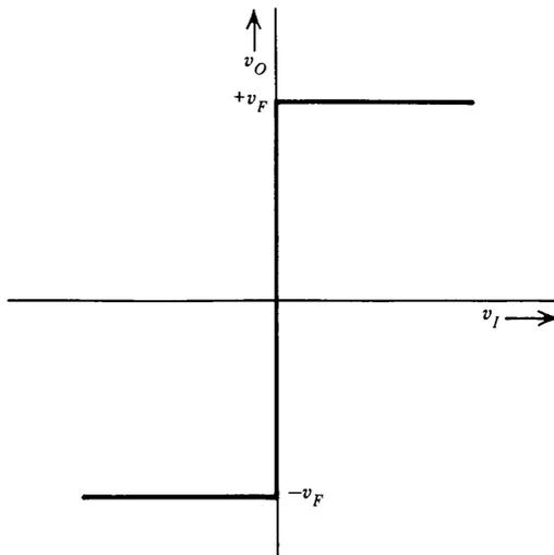
**Figure 12.41** Infinite-gain limiter.
