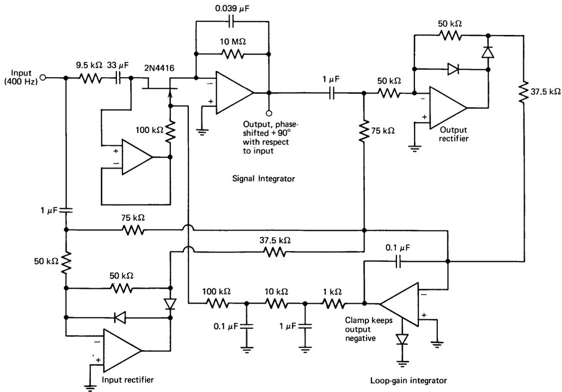
**Figure 12.32** Precision phase shifter with amplitude control.
