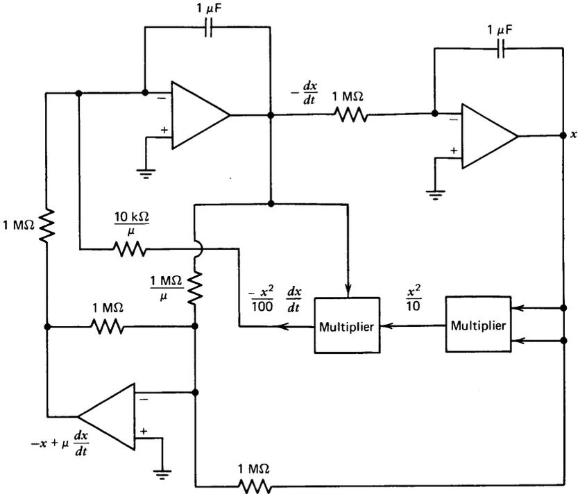
**Figure 12.14** Simulation of Van der Pol's equation.
