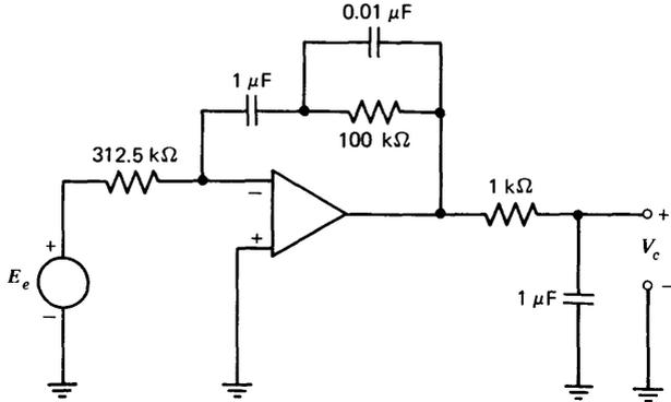
**Figure 12.6** Controller circuit.
