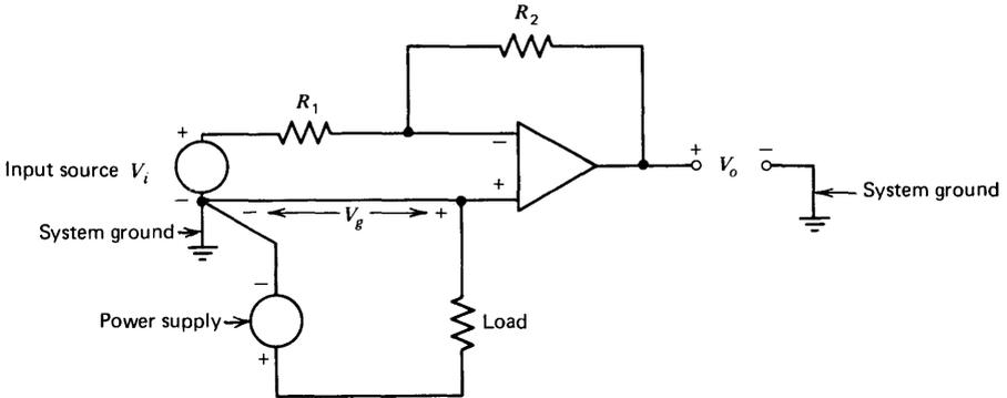
**Figure 11.9** An example of poor grounding technique.
