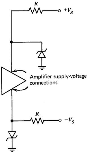
Figure 11.6 Supply-voltage limiting.
