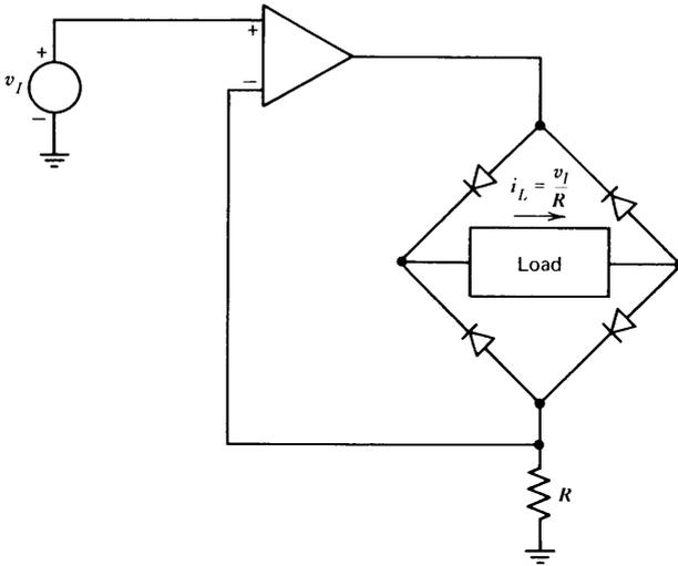
Figure 11.19 Full-wave precision rectifier for floating load.
