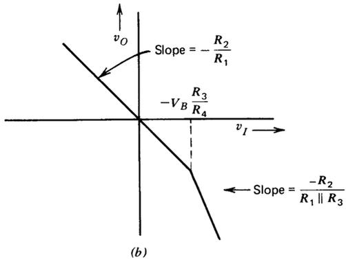
**Figure 11.24** Expander. (a) Circuit. (b) Transfer characteristics.
