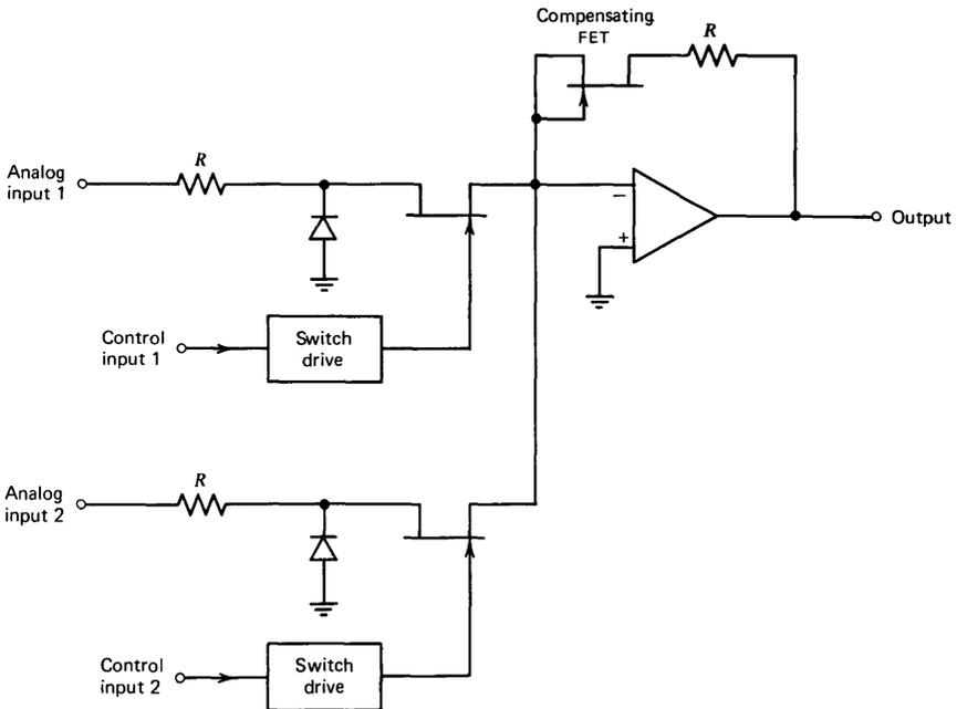
**Figure 11.31** Inverting multiplexer.
