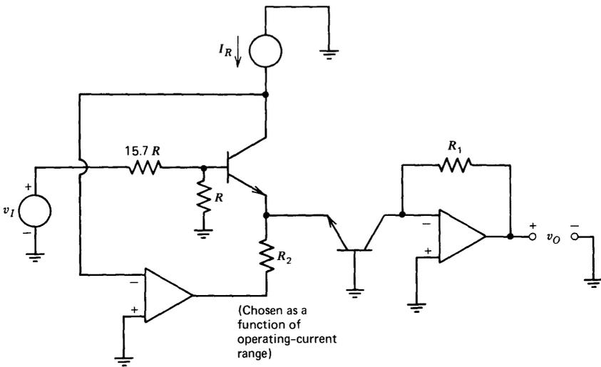
Figure 11.27 Antilog circuit.
