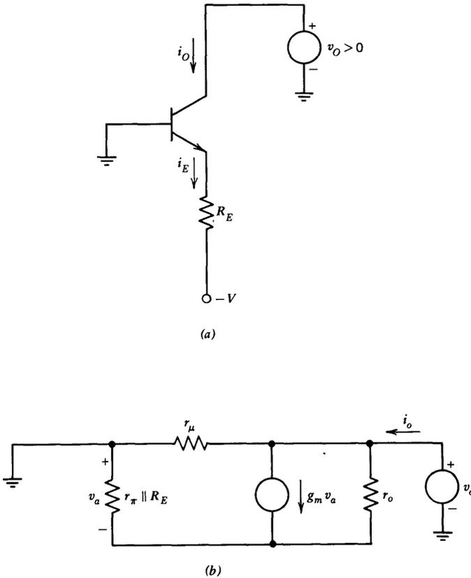
**Figure 8.17** Current source. (a) Schematic. (b) Equivalent circuit.
