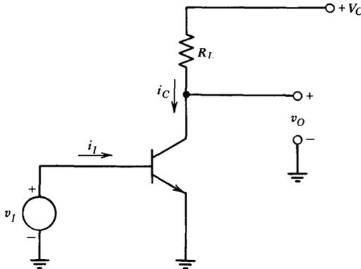
**Figure 8.10** Common-emitter amplifier.
