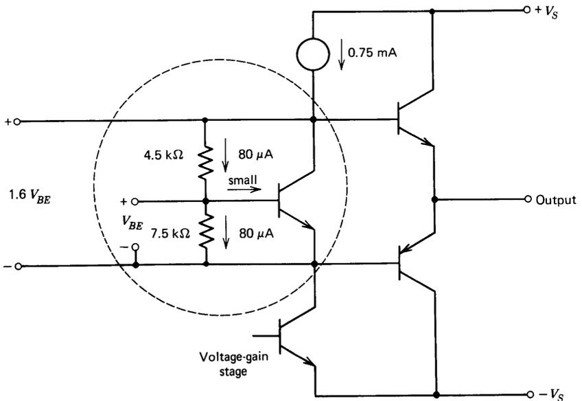
**Figure 8.26** Bias circuit used in 741 amplifier.
