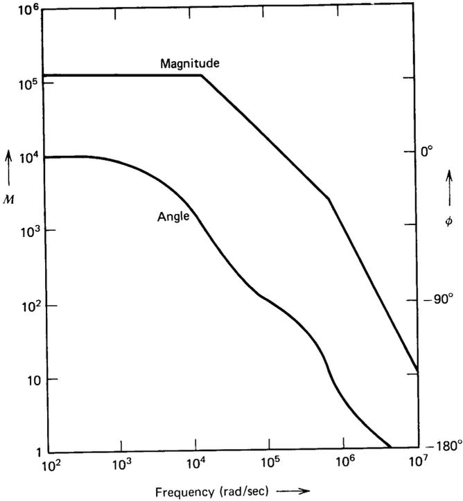
Figure 8.2 Transfer function for amplifier of Fig. 8.1.
