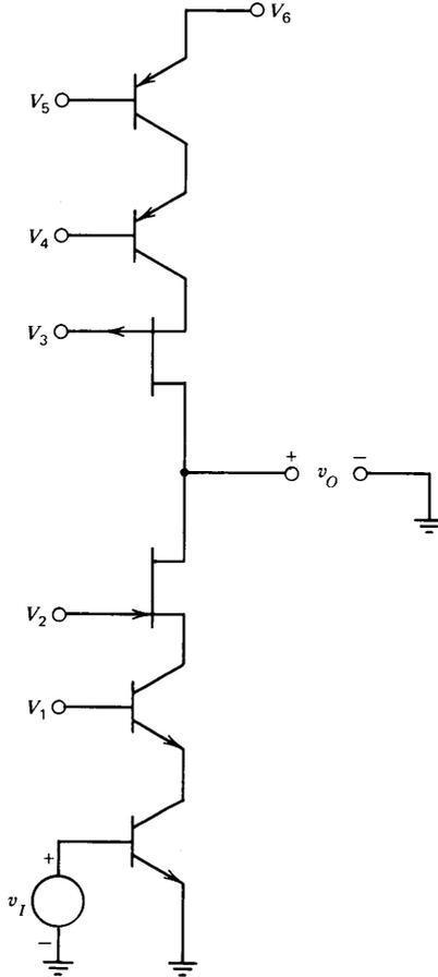
**Figure 8.34** High-gain amplifier.
