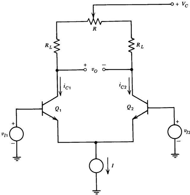
**Figure 7.10** Method for balancing with equal base-to-emitter voltages.
