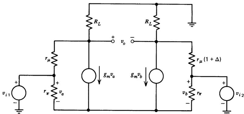
**Figure 7.8** Circuit illustrating effect of unequal  $r_{\mu}$ 's.
