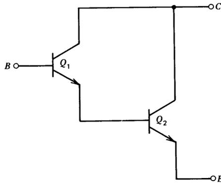
Figure 7.19 Darlington-connected transistors.
