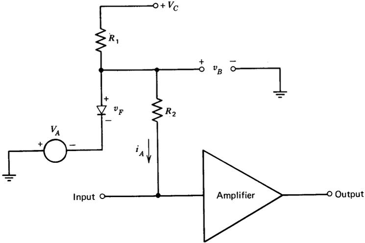
**Figure 7.15** Use of a diode for input-current compensation.
