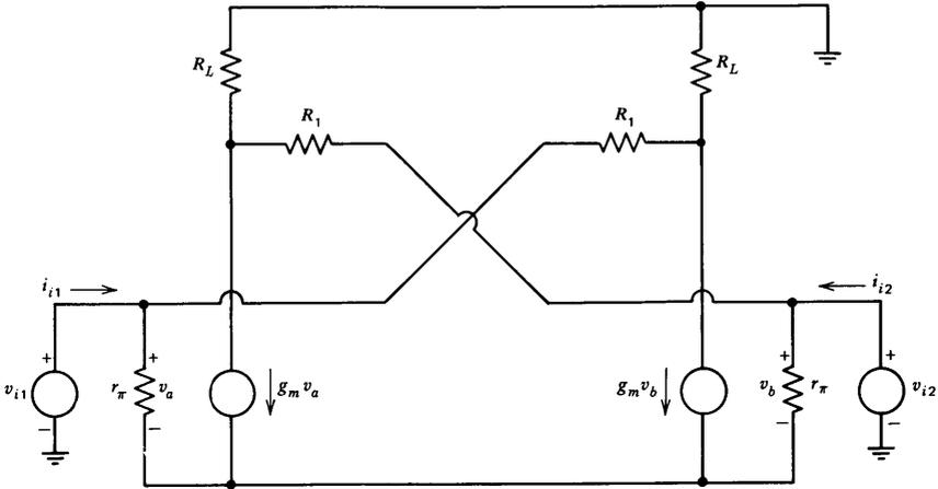
Figure 7.17 Incremental model for circuit of Fig. 7.16.
