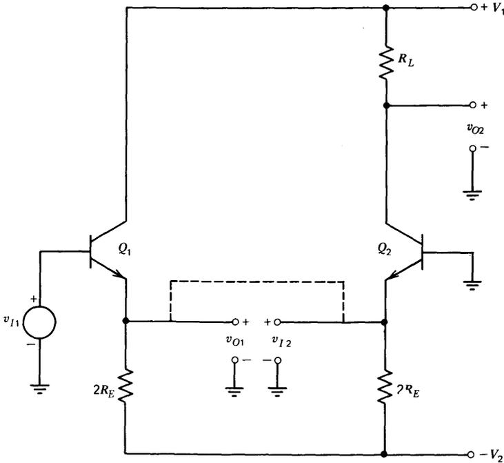
Figure 7.3 Circuit illustrating development of the differential amplifier.
