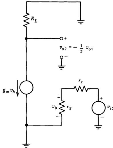
Figure 7.6 Right-hand half circuit for a differential input.
