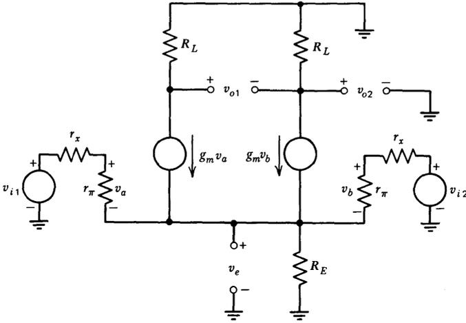
Figure 7.5 Incremental model for a differential amplifier.
