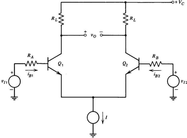
**Figure 7.13** Method to eliminate effects of input current.
