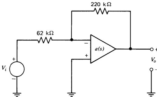
**Figure 5.29** Inverting configuration.
