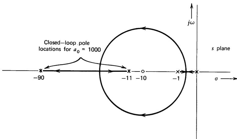
Figure 5.19 Root-locus diagram for  $a(s)f(s) = a_0(0.1s + 1)/[s(s + 1)]$ .
