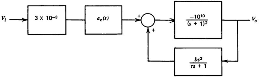
Figure 5.27 Operational-amplifier model.
