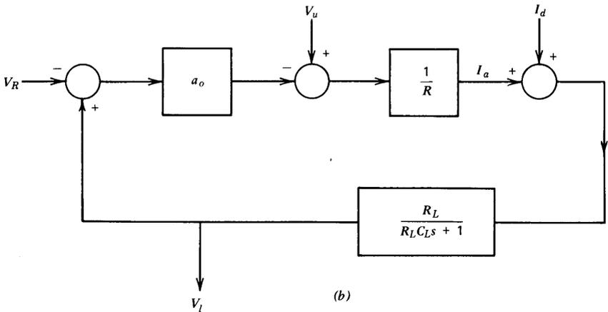
**Figure 5.3** Voltage regulator. (a) Circuit. (b) Block diagram.
