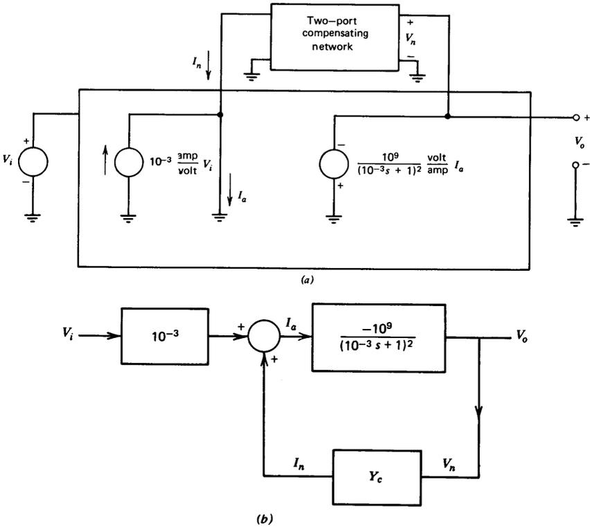
Figure 5.22 Operational amplifier. (a) Model. (b) Block diagram.
