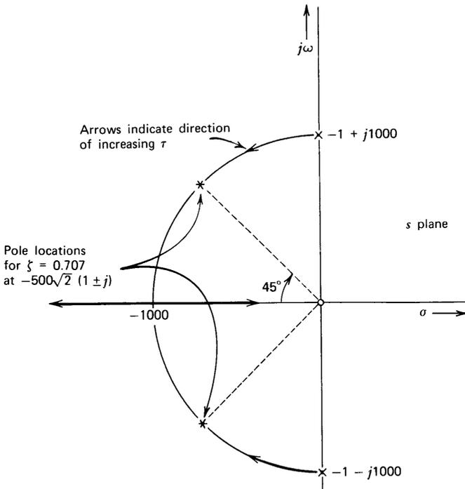
**Figure 4.15** Root-contour diagram for  $p'(s)/q'(s) = 10^6 s / (s^2 + 2s + 10^6)$ .
