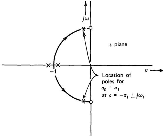
**Figure 4.13** Root-locus diagram for systems of Figs. 4.11 and 4.12.
