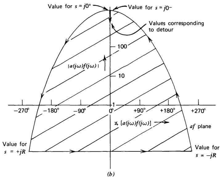
**Figure 4.18** Nyquist test for  $a(s)f(s) = 10^3 / [(s + 1)(0.1s + 1)(0.01s + 1)]$ .
