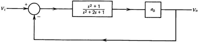
Figure 4.11 Rejection amplifier.
