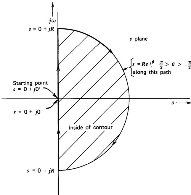
**Figure 4.16** Contour Used to evaluate  $a(s)f(s)$ .
