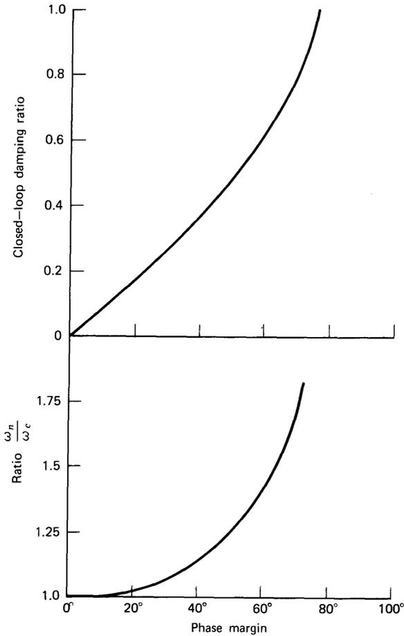
**Figure 4.26a** Closed-loop quantities from loop-transmission parameters for system with two widely spaced poles. Damping ratio and natural frequency as a function of phase margin and crossover frequency.
