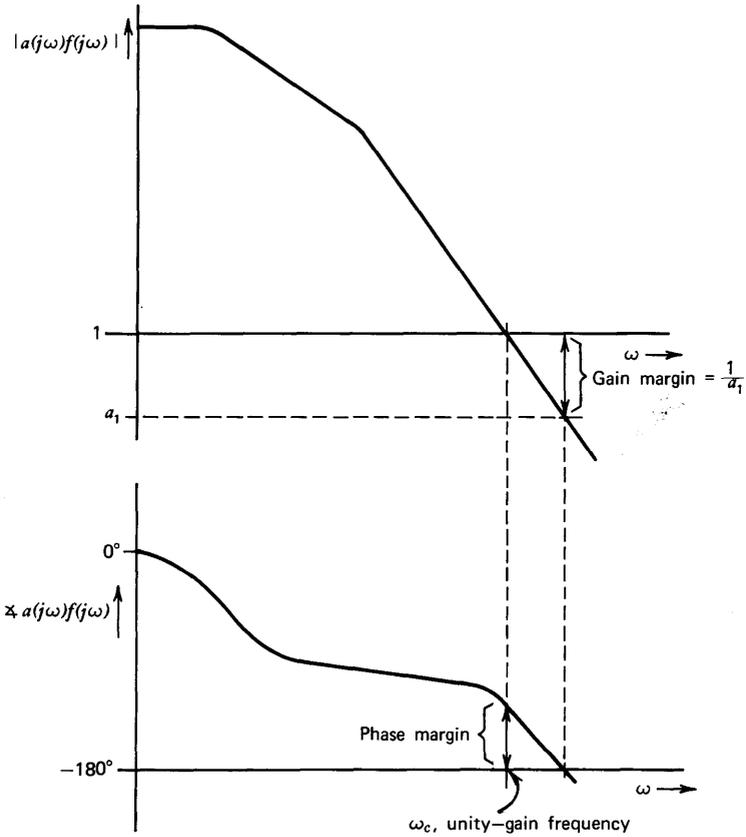
**Figure 4.21** Loop-transmission quantities.
