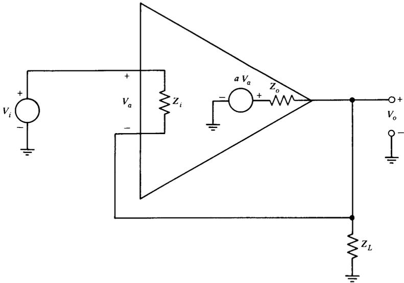
Figure 2.26 Noninverting amplifier.
