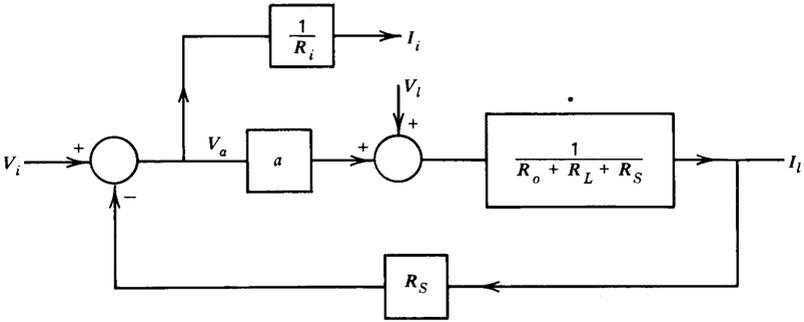
Figure 2.18 Block diagram for amplifier of Fig. 2.17.
