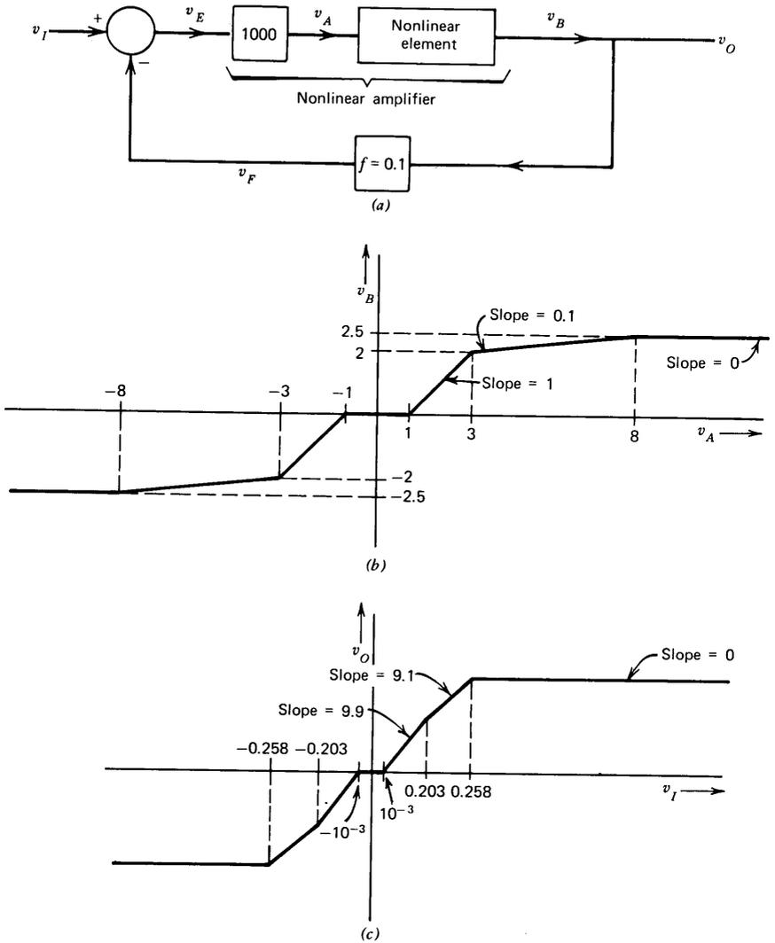
**Figure 2.4** The effects of feedback on a nonlinearity. (a) System. (b) Transfer characteristics of the nonlinear element. (c) System transfer characteristics (closed loop). (Not to scale.) (d) Waveforms for  $v_I(t)$  a unit ramp. (Not to scale.)
