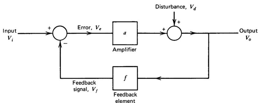
**Figure 2.2** Block diagram for the system of Fig. 2.1.
