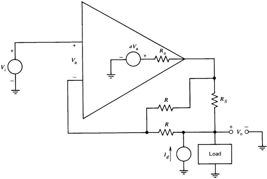
**Figure 2.28** Operational-amplifier connection with controlled output resistance.
