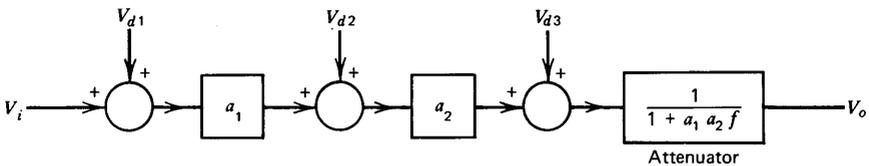
Figure 2.6 Open-loop system illustrating effects of disturbances.
