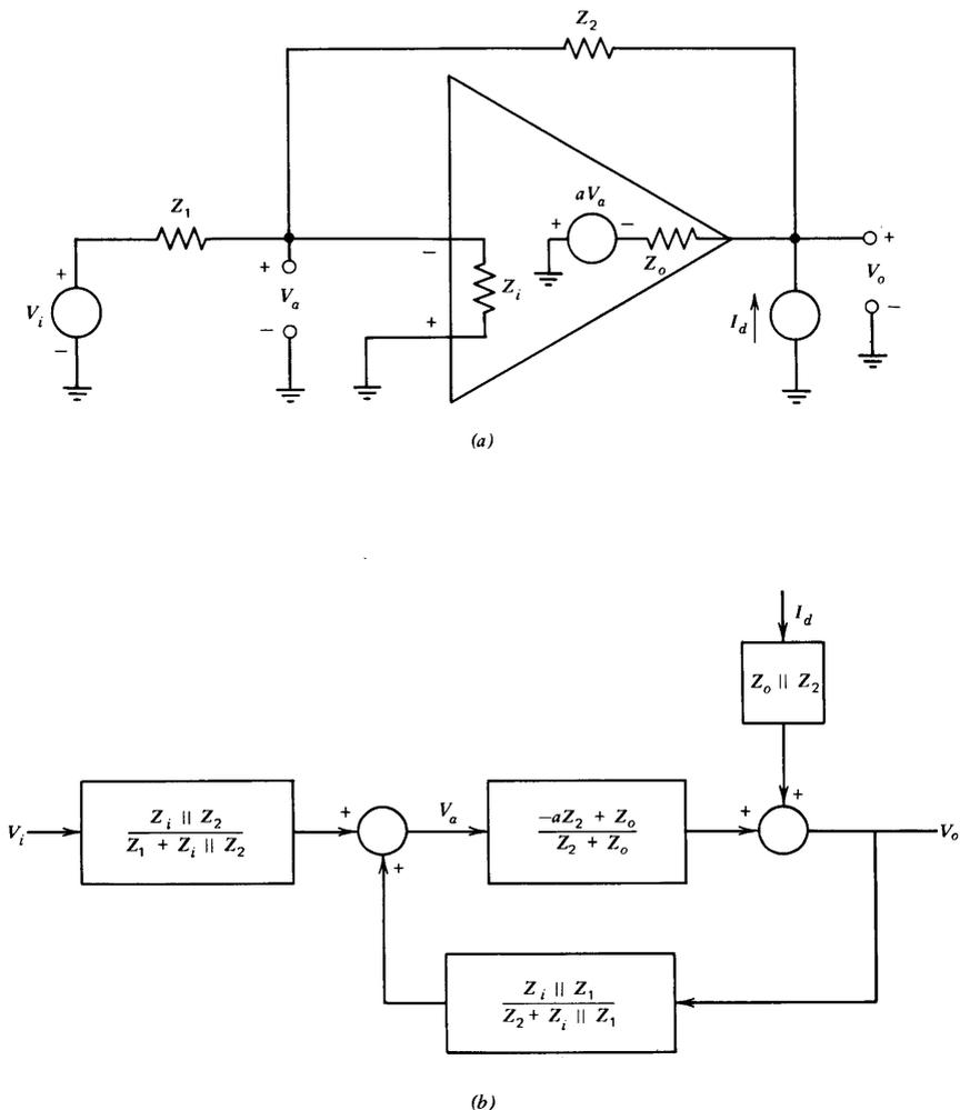
**Figure 2.9** Inverting amplifier. (a) Circuit. (b) Block diagram.
