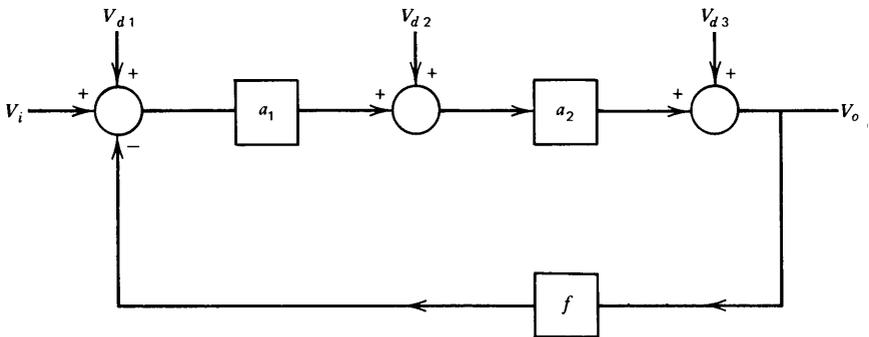
**Figure 2.5** Feedback system illustrating effects of disturbances.
