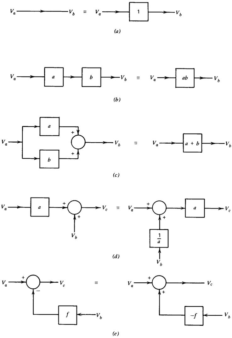
**Figure 2.10** Block-diagram equivalences. (a) Unity gain of line. (b) Cascading. (c) Summation. (d) Absorption. (e) Negation. (f) Branching. (g) Factoring. (h) Loop reduction.
