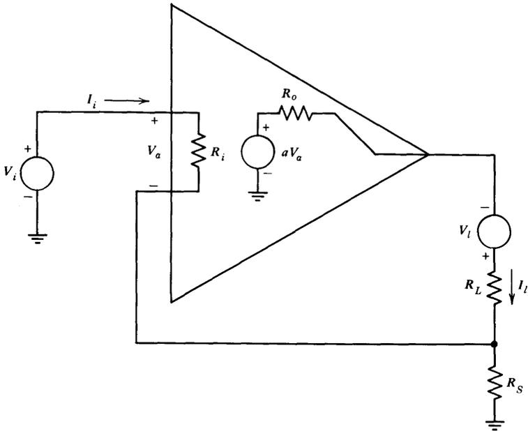
**Figure 2.17** Amplifier with high input and output resistances.
