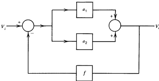
**Figure 2.21** Feedback system with parallel forward paths.
