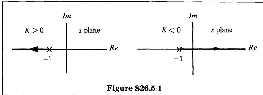
The pole moves from infinity to negative infinity as  $K$  changes from negative infinity to infinity.
