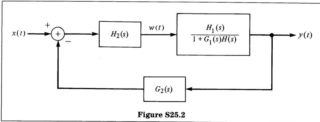
$$\begin{aligned} \frac{Y(s)}{X(s)} &= \frac{\frac{H_1(s)H_2(s)}{1 + G_1(s)H_1(s)}}{1 + \frac{G_2(s)H_1(s)H_2(s)}{1 + G_1(s)H_1(s)}} \\ &= \frac{H_1(s)H_2(s)}{1 + G_1(s)H_1(s) + G_2(s)H_1(s)H_2(s)} \end{aligned}$$
