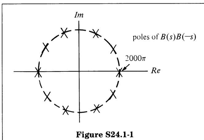
(c) For  $B(s)$  to be stable and causal, its poles must be in the left half-plane, as shown in Figure S24.1-2.
