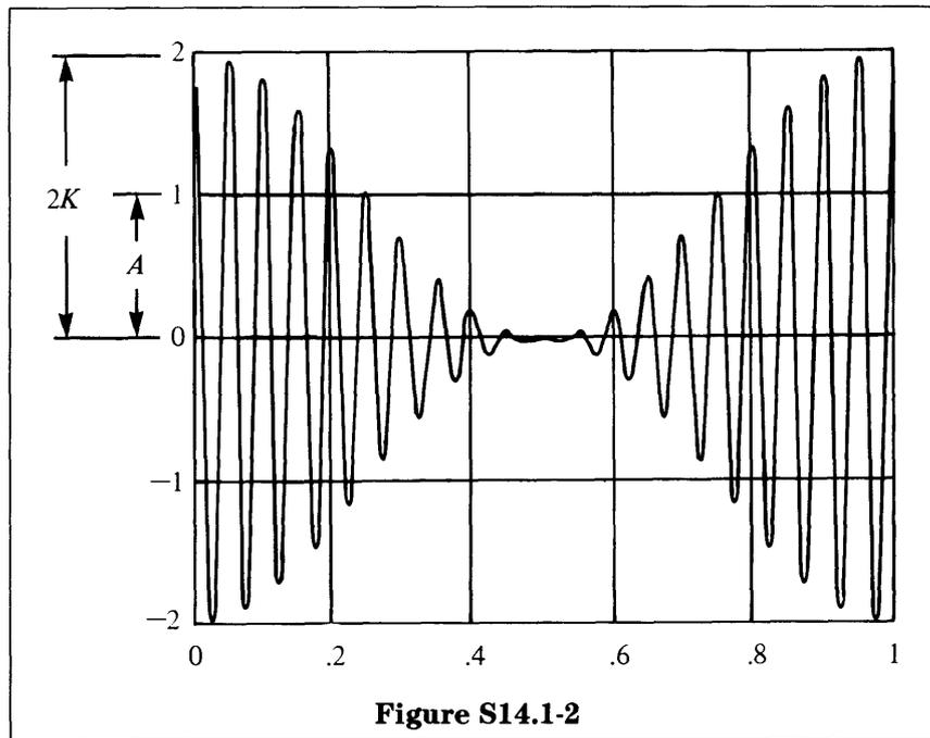
(c)  $2K = 2$ ,  $K = 1$ ,  $A = 0.5$ , so  $K/A = 2$ , and the signal has 200% modulation.
