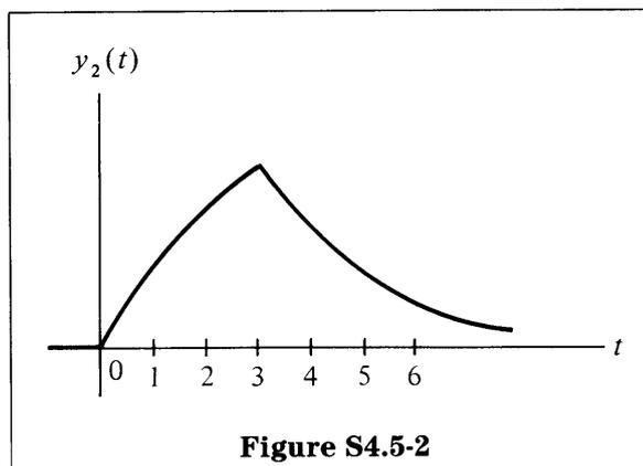
(b) Since  $x_2(t) = 2[x_1(t) - x_1(t - 3)]$  and the system is linear and time-invariant,  $y_2(t) = 2[y_1(t) - y_1(t - 3)]$ .
