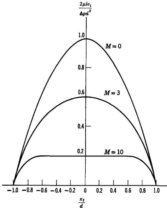
Fig. 14.2.6 Variation of velocity profile with Hartmann number.
