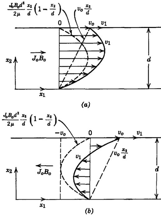
Fig. 14.2.2 Velocity profiles resulting from uniform magnetic force density applied to shear flow. The profiles are sketched for  $|J_o B_o| = 8\mu v_o/d^2$ : (a)  $J_o B_o > 0$ ,  $\mathbf{J} \times \mathbf{B}$  force density is in direction of  $v_o$ ; (b)  $J_o B_o < 0$ ,  $\mathbf{J} \times \mathbf{B}$  force density is opposite to  $v_o$ .
