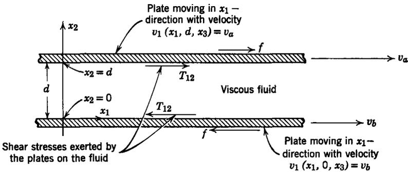
Fig. 14.1.1 Simple example of shear flow.
