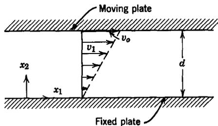
Fig. 14.1.12 A simple example of shear flow.
