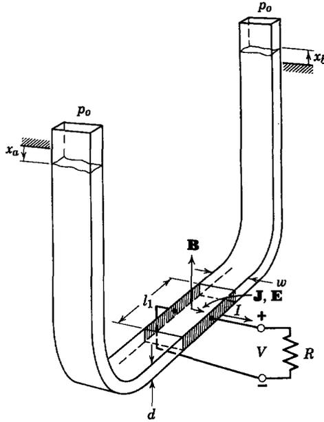
Fig. 12.2.8 Transient-flow problem with electromechanical coupling.
