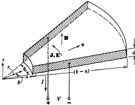
Fig. 12.2.11 MHD conduction machine with variable area.
