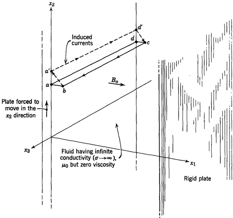
**Fig. 12.2.14** Fluid contained between rigid parallel plates and immersed in a magnetic induction  $B_0$ . Motions of the fluid are induced by transverse motions of the left-hand plate, which, like the fluid, is assumed to be highly conducting.
