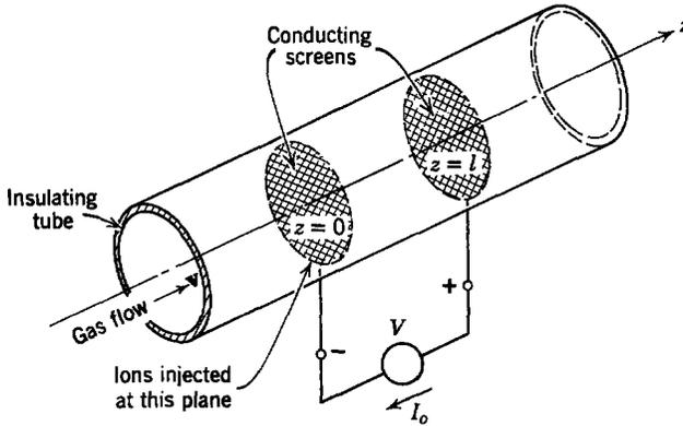
Fig. 12.3.1 Configuration for a gaseous electrostatic pump or generator.
