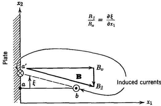
**Fig. 12.2.15** End view of the loop  $abcd$  shown in Fig. 12.2.14. The initial loop formed by conducting fluid and the plate links zero flux  $\lambda$ . To conserve the flux, density  $\mathbf{B}$  remains tangential to the loop with the additional magnetic flux density  $B_2$  created by an induced current.
