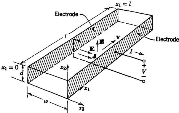
**Fig. 12.2.3** Conduction-type, MHD machine.
