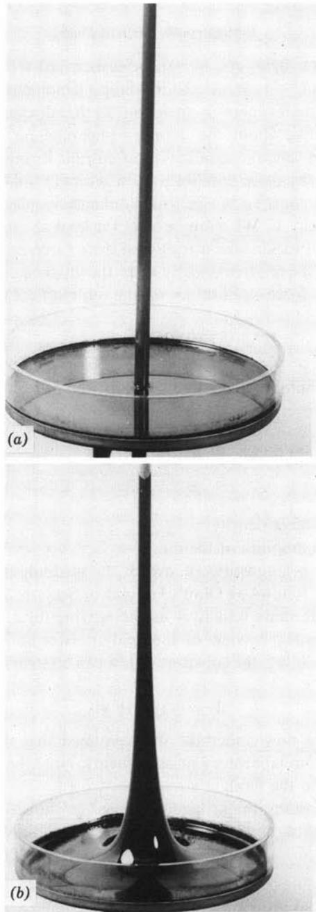
**Fig. 12.2.24** (a) A conductor passes along the axis of symmetry through a pan containing the magnetizable liquid,  $I = 0$ . (b) The current  $I$  has been turned on. The result is a force density  $-\mathbf{H} \cdot \mathbf{H} \nabla \mu$  that tends to lift the fluid upward, as predicted by (12.2.137). (Courtesy of AVCO Corporation, Space Systems Division.)
