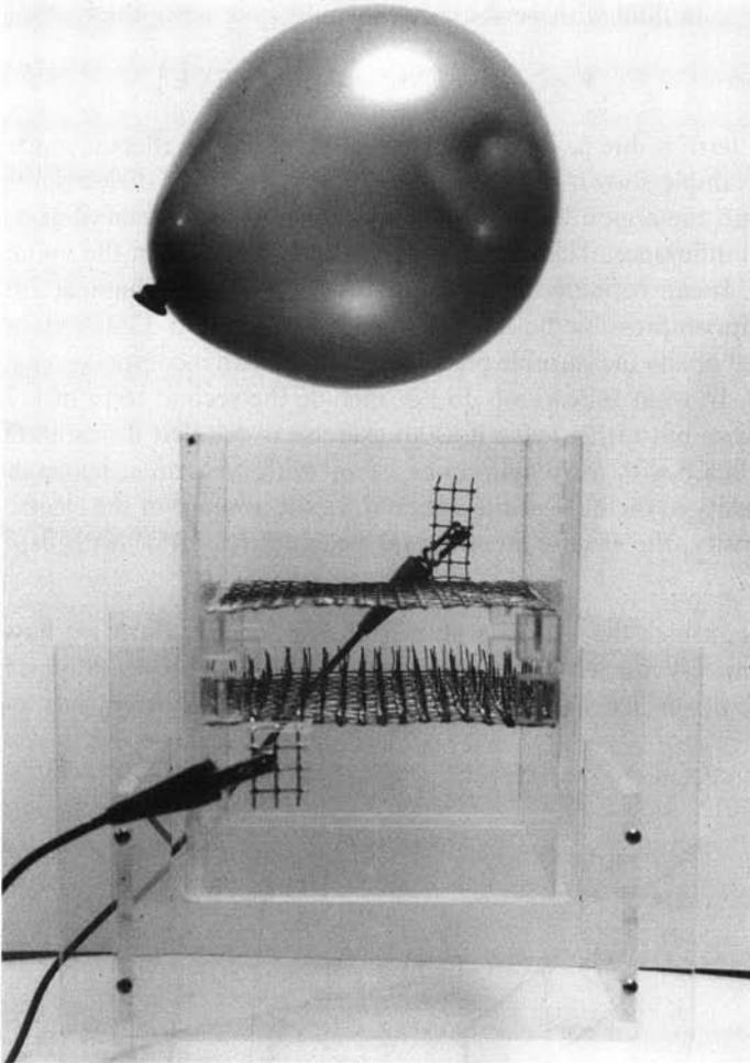
**Fig. 12.3.4** Simple laboratory demonstration of ion-drag effect. In the absence of an applied voltage the balloon rests on the plastic enclosure. With voltage, it is pushed upward by ions being conducted between the grids.
