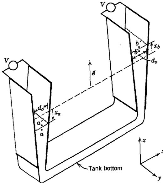
**Fig. 12.3.5** A liquid pendulum containing dielectric fluid. Slightly diverging plates are used to impose a spatially varying electric field that tends to maintain the liquid in the bottom of the tank in spite of the acceleration  $g$ .
