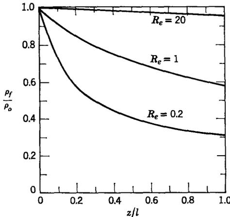
Fig. 12.3.2 Charge-density distribution between grids.  $J/\rho_o v_o = 1$ .
