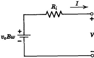
Fig. 12.2.4 Electrical equivalent circuit of conduction-type MHD machine.
