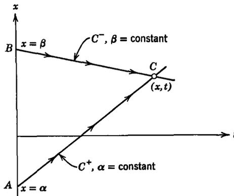
Fig. 10.2.3 Characteristics that intersect at a general point in space and time  $(x, t)$  showing the points  $A$  and  $B$  at which the initial conditions determine the dependent variables at  $C$ .
