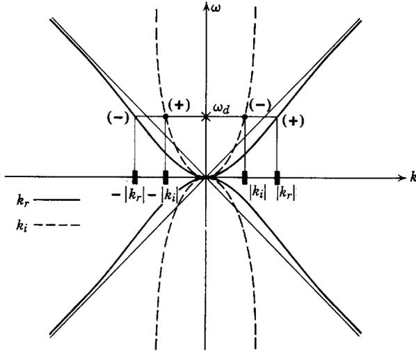
**Fig. 10.1.17** Dispersion equation (10.1.37) for a string immersed in a viscous liquid, showing complex values of  $k$  for real values of  $\omega$ .
