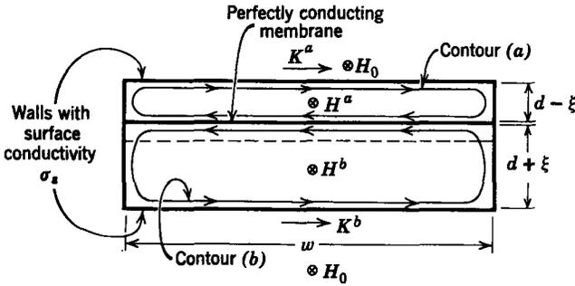
**Fig. 10.1.8** Cross-sectional view of the apparatus shown in Fig. 10.1.7. The current loops (a) and (b), with the imposed magnetic field  $H_0$ , couple the membrane to the upper and lower conducting walls.
