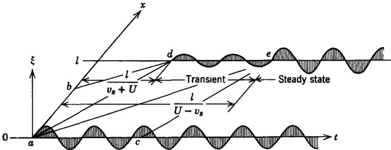
**Fig. 10.2.7** A sinusoidal excitation turned on at  $x = 0$  when  $t = 0$  is applied to a moving string ( $U > v_s$ ). At the downstream position  $x = l$  the sinusoidal steady state is established when the slow wave arrives [ $t = l/(U - v_s)$ ].
