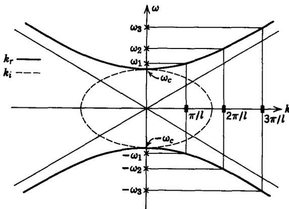
Fig. 10.1.6 A dispersion equation for waves on the wire in Fig. 10.1.2 showing the relationship between the eigenfrequencies  $\omega_n$  and the eigenvalues  $k = n\pi/l$ .
