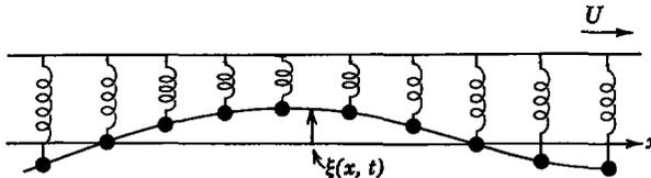
**Fig. 10.2.11** When  $f \rightarrow 0$  ( $v_s \rightarrow 0$ ), the moving string subject to the restoring force of the magnetic field is equivalent to a distribution of mass-spring oscillators with the resonance frequency  $\omega_c$  and moving with the velocity  $U$  in the  $x$ -direction.
