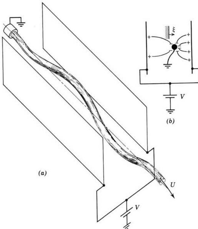
**Fig. 10.2.15** (a) A jet of water has a streaming velocity  $U$  midway between plane-parallel electrodes. A potential difference  $V$  is applied between the plates and the jet. (b) As the jet is deflected toward one of the plates, an unbalance in the electric force of attraction tends to carry it even farther in the direction of deflection. The instability resulting from this force is washed downstream to form the convective instability sketched in Fig. 10.2.16.
