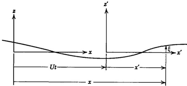
**Fig. 10.2.1** The fixed coordinate system  $x, y, z$  or the moving coordinate system  $x', y', z'$  can be used to define a given position along the equilibrium axis of the string. Because the moving coordinate system has the same velocity  $U$  in the  $x$ -direction as the string, the string appears to move only in the  $z'$ -direction when viewed from the primed frame.
