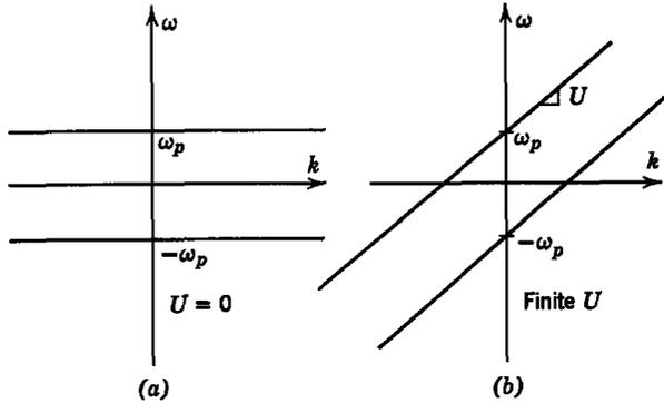
Fig. 10.2.12 Dispersion plot for electron oscillations having the plasma frequency  $\omega_p$ : (a) the electrons with a fixed equilibrium state; (b) electrons with an equilibrium velocity  $U$  in the  $x$ -direction.
