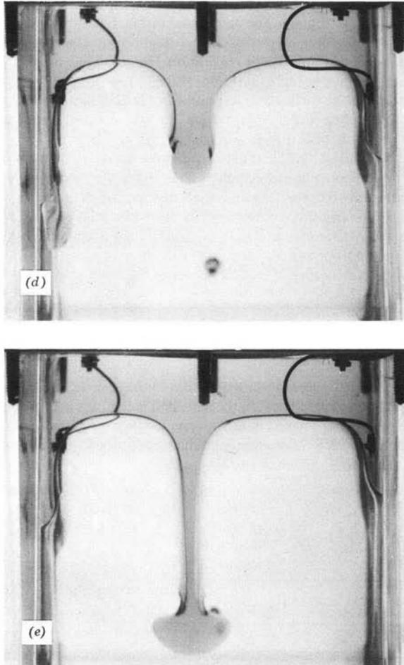
**Fig. 10.1.13** (a) A heavy (dark) liquid is supported above a light (clear) liquid by hydrostatic pressure; (b - e) show growth of Rayleigh-Taylor instability resulting after stabilizing electric polarization forces in (a) are removed. (Photograph courtesy of Dynatech Corp., Cambridge, Mass.) This phenomenon can be seen in the film, "Complex Waves II," available from Education Development Center, Inc., Newton, Mass.
