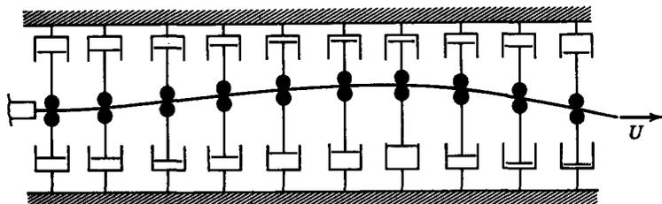
Fig. 10.2.17 The string moves unimpeded in the  $x$ -direction with the velocity  $U$ , and transverse motions are retarded by dashpots that interact with the string through rollers. The dashpots are fixed to the laboratory frame of reference.
