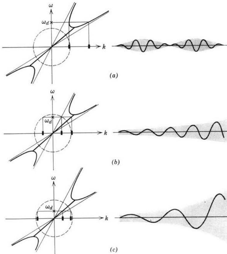
**Fig. 10.2.16** Sinusoidal excitation of jet shown in Fig. 10.2.15. Driving frequency decreases from (a) to (c). This experiment together with animated  $\omega$ - $k$  plots can be seen in the film "Complex Waves II," produced for the National Committee on Electrical Engineering Films by the Education Development Center, Newton, Mass.
