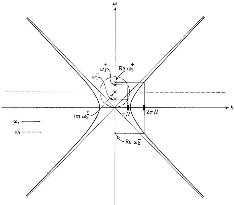
**Fig. 10.1.19** Dispersion equation for string in a viscous liquid showing complex values of  $\omega$  for real values of  $k$ . The lowest pairs of eigenfrequencies for a string fixed at each end are shown.
