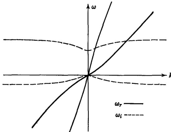
**Fig. 10.2.18** Dispersion equation for resistive wall instability. Complex values of  $\omega$  are shown for real values of  $k$ . Although this plot indicates that the string deflections are unstable, the instability is exhibited as a growth in space rather than in time.
