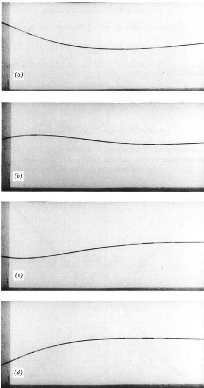
**Fig. 10.1.18** A spring under tension is driven sinusoidally at the left end and fixed at the right end. It is immersed in glycerine which is sufficiently viscous that the effect of damping exceeds that of inertia. Hence the resulting motions which are shown in sequence over about one half cycle exemplify diffusion waves (or skin effect waves) in the sinusoidal steady state. (From four-minute film "Diffusion Waves" made for M.I.T. by Education Development Center, Inc., Newton, Mass.)
