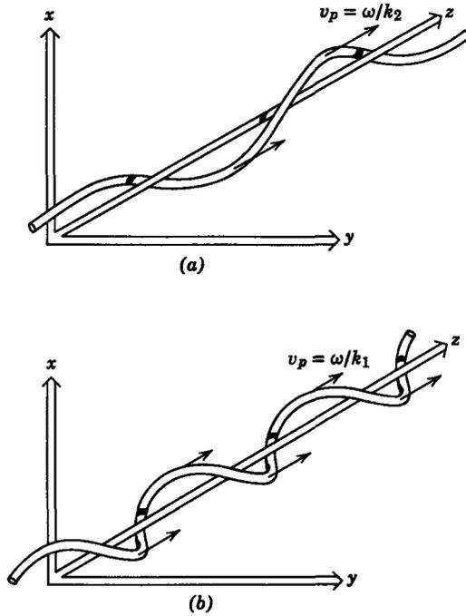
**Fig. 10.4.6** Waves propagating in the  $+z$ -direction: (a) fast wave with a wavelength  $2\pi/k_2$ ; and (b) slow wave with a wavelength  $2\pi/k_1$ .
