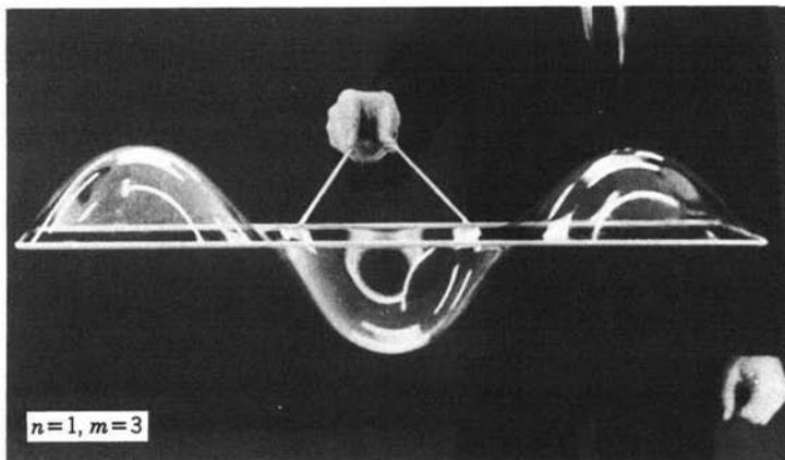
**Fig. 10.4.2** Membrane motions illustrated by soap film on a vibrating wire frame. Pictures from film "Soap Film Oscillations." Courtesy of A. M. Hudson, Occidental College and Film Studio, Education Development Center, Inc., Newton, Mass.
