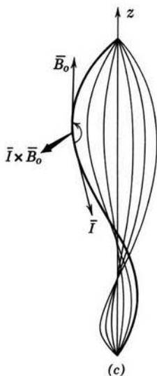
**Fig. 10.4.7** (a) Experiment in which a conducting spring is stretched between pole faces of a magnet. There is a vertical field  $B_0$  and a current has just been applied to the spring. (b) A moment later instability occurs. (c) Predicted  $n = 1$  mode at point of impending instability. (From Film "Complex Waves I, Propagation, Evanescence and Instability," produced by Education Development Center, Inc., Newton, Mass., for the National Committee on Electrical Engineering Films.)
