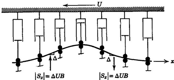
**Fig. 10.2.20** A pulse is initially stationary when viewed from a frame moving with the string. Then, as the dashpots move to the left, they produce a force with a sign determined by the slope of the string.
