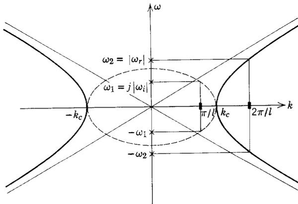
**Fig. 10.1.11** The dispersion equation for the system of Fig. 10.1.2 with current as shown in Fig. 10.1.9. Complex values of  $\omega$  are shown for real values of  $k$ . The allowed values of  $k$  give rise to the eigenfrequencies as shown.
