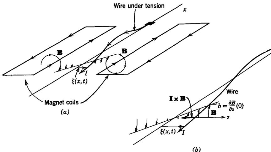
Fig. 10.1.2 (a) A conducting wire is stretched along the  $x$ -axis and is free to undergo transverse motions in the horizontal plane. Magnet coils produce a field  $\mathbf{B}$  which is zero along the  $x$ -axis; (b) the wire carries a current  $I$  so that deflections from the  $x$ -axis result in a force that tends to restore the wire to its equilibrium position.
