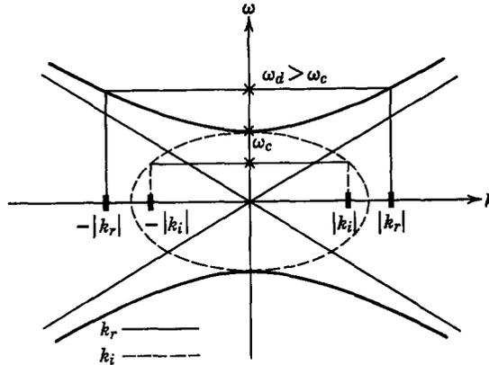
Fig. 10.1.3 Dispersion relation for the wire subject to a restoring force distributed along its length (for the case shown in Fig. 10.1.2). Complex values of  $k$  are shown as functions of real values of  $\omega$ .
