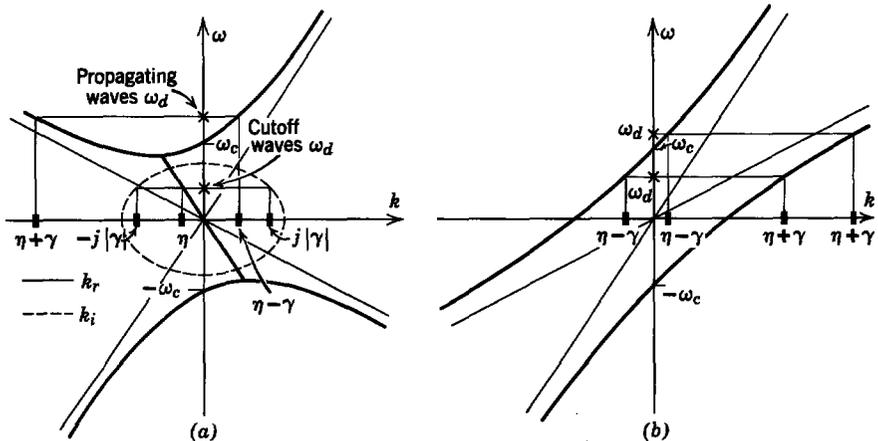
Fig. 10.2.10 Dispersion relations for system of Section 1.2, with the addition of a longitudinal velocity  $U$ . When  $U$  exceeds  $v_s$ , both waves propagate without decay, regardless of the frequency, and the effect of the convection is to eliminate the evanescence. (a)  $U < v_s$ ; (b)  $U > v_s$ .
