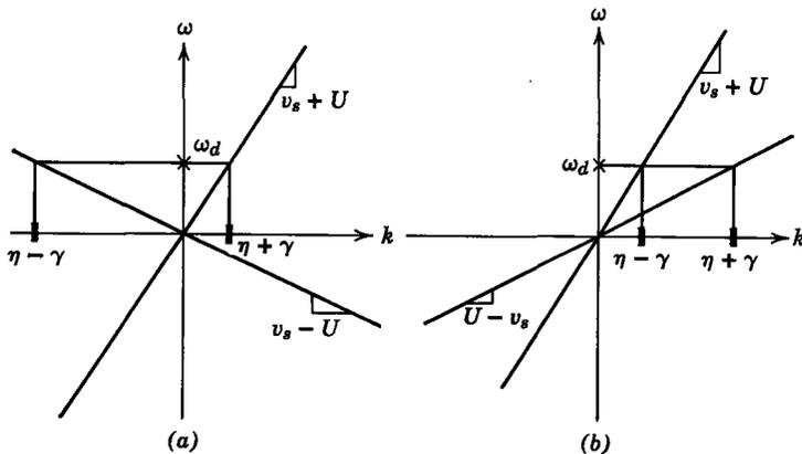
Fig. 10.2.8 Dispersion relations for waves on a string moving with the equilibrium velocity  $U$  in the positive  $x$ -direction. Although the geometry for the subsonic and supersonic cases is the same as that for the characteristic lines in Fig. 10.2.2, the axes here are  $\omega$ - $k$ , whereas in Fig. 10.2.2 they are  $x$ - $t$ : (a)  $U < v_s$ ; (b)  $U > v_s$ .
