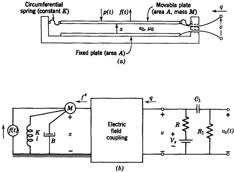
**Fig. 5.1.11** Electric field transducer that can be used as a pressure sensor (microphone) or pressure source (speaker): (a) cross section of device (side view); it would appear circular from above; (b) equivalent electromechanical circuit.
