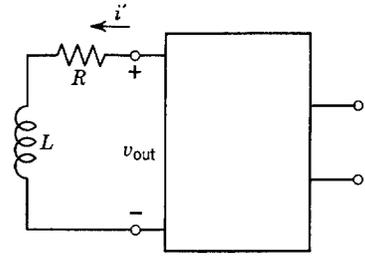
**Fig. 5.1.9** The driving current of Fig. 5.1.8a is produced by a voltage amplifier connected in series with a large resistance  $R$ . The output voltage is proportional to the displacement  $x'$ . The inductance  $L$  is the equilibrium inductance of the coil shown in Fig. 5.1.8a.
