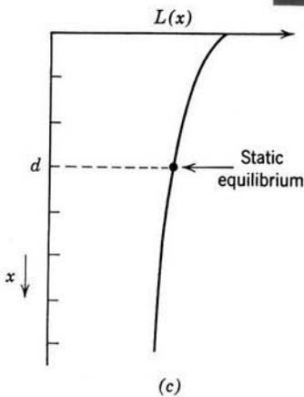
**Fig. 5.1.8** (a) Mass  $M$  levitated by a magnetic field. The optical system provides a signal that is fed back to stabilize the static equilibrium of the mass at  $x = d$ ; (b) view of laboratory project shown schematically by (a); (c) dependence of coil inductance on the mass displacement.
