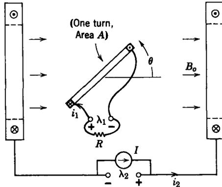
Fig. 5.1.14 A pivoted coil is free to rotate with the angular deflection  $\theta$  in a uniform magnetic field produced by  $i_2$ .
