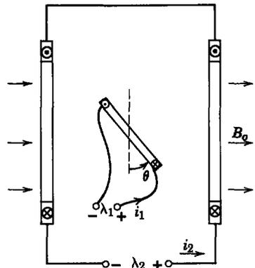
**Fig. 5.2.4** A pair of fixed coils is excited in series by the current  $i_2$ . A pivoted coil has the angular deflection  $\theta$  and the electrical terminal variables  $(i_1, \lambda_1)$ . When both coils are driven by constant current sources, the potential well is as shown in Fig. 5.2.2.
