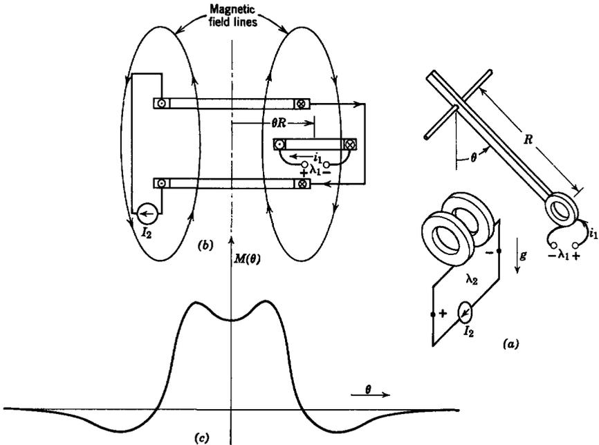
**Fig. 5.2.5** (a) A coil is attached to a pendulum in such a way that when  $\theta = 0$  it is directly between a pair of fixed coils energized by the current  $I_2$ ; (b) top view of (a) showing the magnetic field produced by the fixed coils; (c) mutual inductance between the fixed and movable coils of (b).
