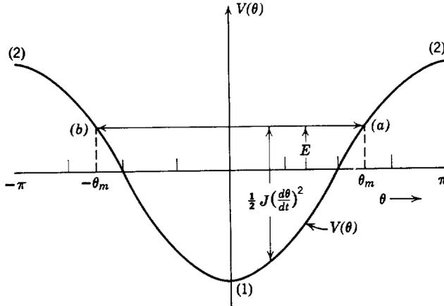
**Fig. 5.2.2** Potential well  $V(\theta)$  for the pendulum of Fig. 5.2.1 and for the rotatable coil of Fig. 5.2.4. If the pendulum is released from a stationary state at  $\theta = \theta_m$ , it will have an excursion between the points (a) and (b). The square of the angular velocity at any given position is proportional to the vertical distance between the constant  $E$  line and the potential  $V(\theta)$ .
