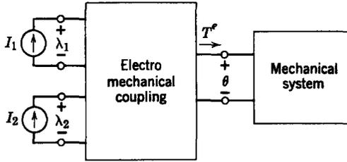
**Fig. 5.2.3** Electromechanical system in which conservation of an energy function can be used to determine the dynamics. The mechanical system is composed of lossless elements and one of each of the electrical terminal variables is held constant.
