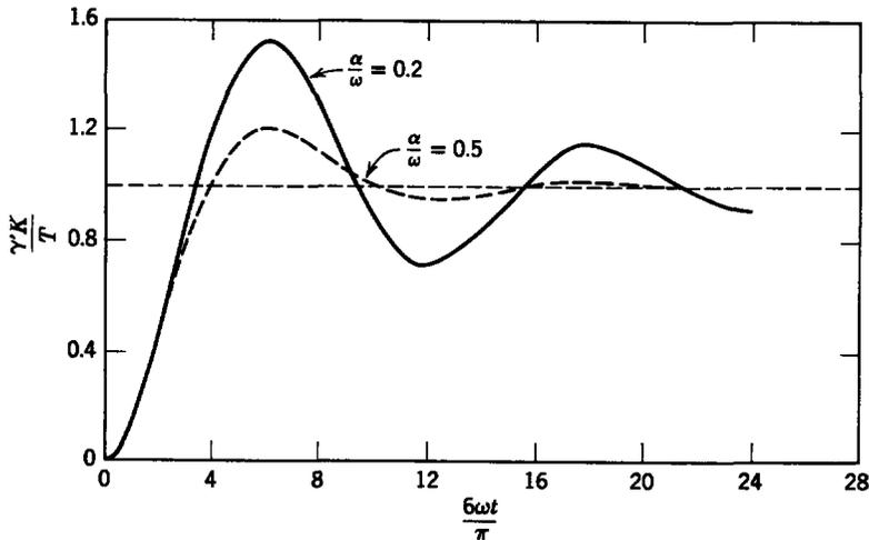
Fig. 5.1.6 Hunting transient of a synchronous machine.
