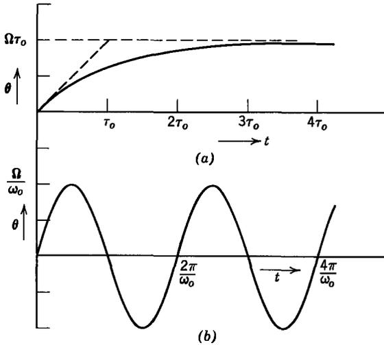
Fig. 5.1.15 Response in angular deflection of the rotatable coil of Fig. 5.1.14 to an initial angular velocity  $\Omega$  at  $\theta = 0$ : (a) motion dominated by electrical resistance ( $\tau_o \gg L_1/R$ ); (b) flux  $\lambda_1$  conserved at zero ( $2\pi/\omega_o \ll L_1/R$ ) as it would be if the resistance  $R$  were very small.
