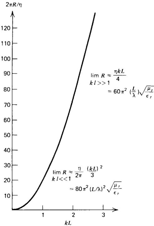
Figure 9-14 The radiation resistance for a dipole antenna carrying a uniformly distributed current increases with the square of its length when it is short ( $L/\lambda \ll 1$ ) and only linearly with its length when it is long ( $L/\lambda \gg 1$ ). For short lengths, the radiation resistance approximates that of a point dipole.
