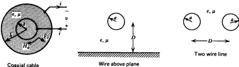
Figure 8-3 Various types of simple transmission lines.
