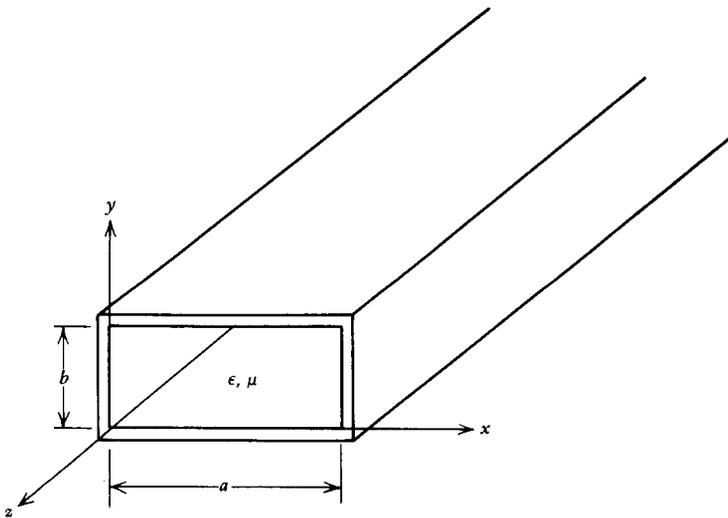
Figure 8-27 A lossless waveguide with rectangular cross section.
