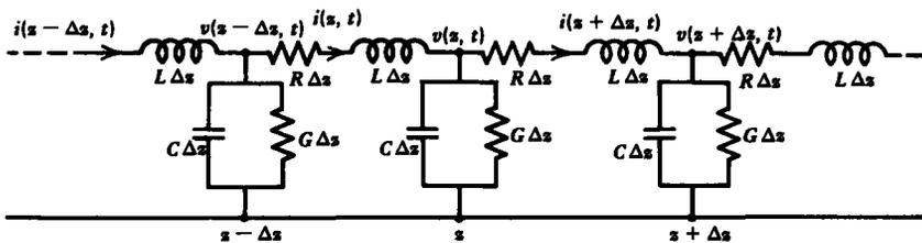
$$v(z, t) - v(z + \Delta z, t) = L \Delta z \frac{\partial}{\partial t} i(z + \Delta z, t) + i(z + \Delta z, t) R \Delta z$$
