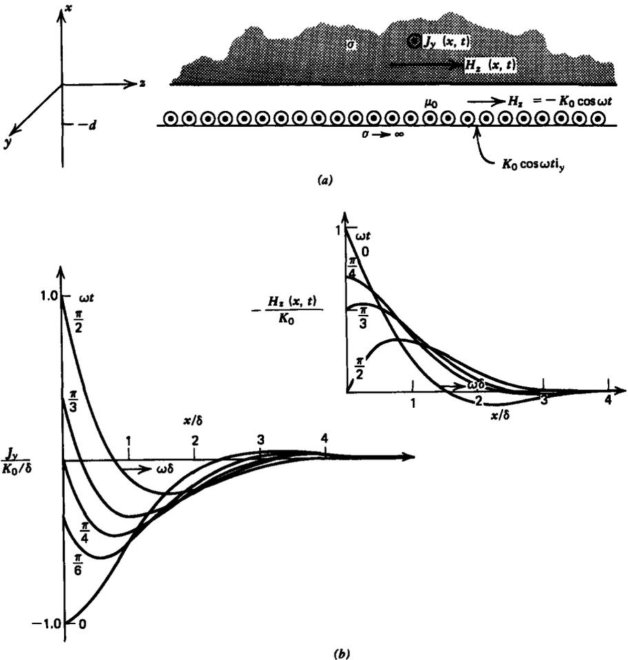
Figure 6-27 (a) A stationary conductor lies above a sinusoidal surface current placed upon a perfect conductor so that  $\mathbf{H} = 0$  for  $x < -d$ . (b) The magnetic field and current density propagates and decays into the conductor with the same characteristic length given by the skin depth  $\delta = \sqrt{2/(\omega\mu\sigma)}$ . The phase speed of the wave is  $\omega\delta$ .
