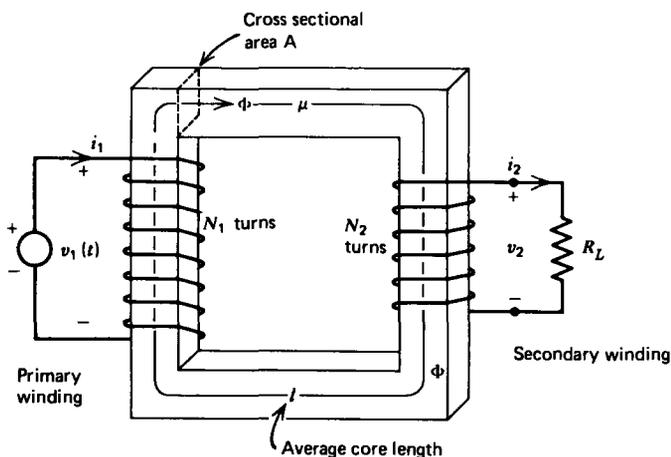
$$\left. \begin{aligned} \frac{v_1}{v_2} &= \frac{N_1}{N_2} \\ \frac{i_1}{i_2} &= \frac{N_2}{N_1} \end{aligned} \right\} \Rightarrow v_1 i_1 = v_2 i_2$$
