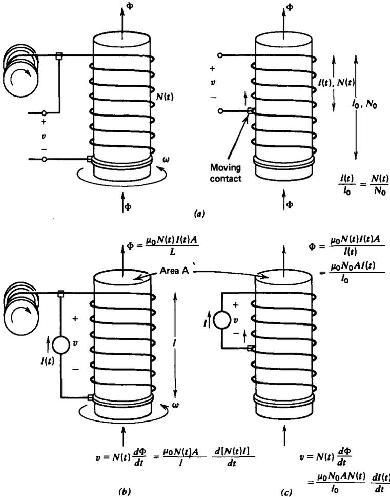
Figure 6-24 (a) If the number of turns on a coil is changing with time, the induced voltage is  $v = N(t) d\Phi/dt$ . A constant flux does not generate any voltage. (b) If the flux itself is proportional to the number of turns, a dc current can generate a voltage. (c) With the tap changing coil, the number of turns per unit length remains constant so that a dc current generates no voltage because the flux does not change with time.
