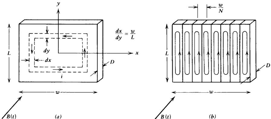
Figure 6-6 (a) A time varying magnetic field through a conductor induces eddy currents that cause Ohmic heating. (b) If the conductor is laminated so that the induced currents are confined to thin strips, the dissipated power decreases.
