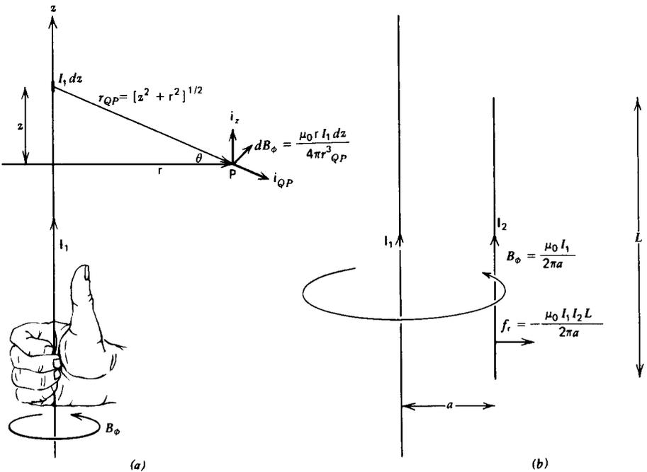
Figure 5-8 (a) The magnetic field due to an infinitely long  $z$ -directed line current is in the  $\phi$  direction. (b) Two parallel line currents attract each other if flowing in the same direction and repel if oppositely directed.
