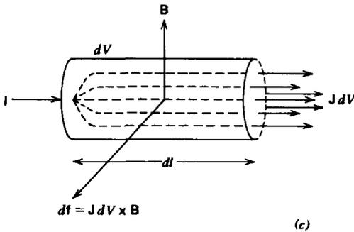
Figure 5-2 Moving line, surface, and volume charge distributions constitute currents. (a) In metallic wires the net charge is zero since there are equal amounts of negative and positive charges so that the Coulombic force is zero. Since the positive charge is essentially stationary, only the moving electrons contribute to the line current in the direction opposite to their motion. (b) Surface current. (c) Volume current.
