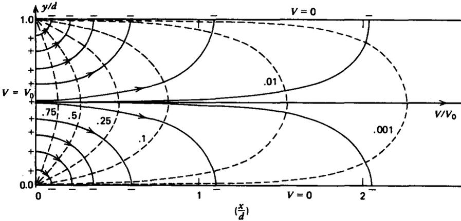
Figure 4-5 An open conducting box of infinite extent in the  $x$  and  $z$  directions and of finite width  $d$  in the  $y$  direction, has zero potential on all surfaces except the closed end at  $x=0$ , where  $V=V_0$ .
