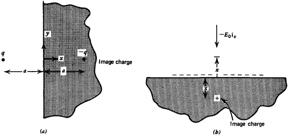
Figure 2-28 (a) A point charge  $q$  near a conducting plane has its image charge  $-q$  symmetrically located behind the plane. (b) An applied uniform electric field causes a uniform surface charge distribution on the conducting plane. Any injected charge must overcome the restoring force due to its image in order to leave the electrode.
