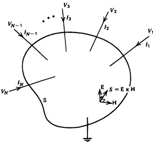
Figure 7-2 The circuit power into an  $N$  terminal network  $\sum_{k=1}^N V_k I_k$  equals the electromagnetic power flow into the surface surrounding the network,  $-\oint_S \mathbf{E} \times \mathbf{H} \cdot d\mathbf{S}$ .
