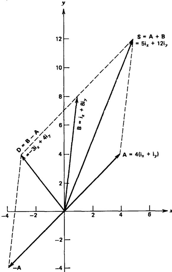
Figure 1-6 The sum and difference of vectors  $A$  and  $B$  given in Example 1-1.
