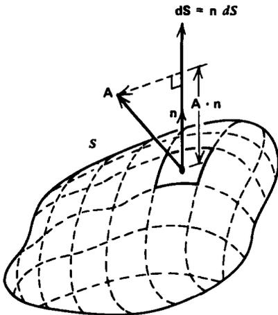
Figure 1-14 The flux of a vector  $\mathbf{A}$  through the closed surface  $S$  is given by the surface integral of the component of  $\mathbf{A}$  perpendicular to the surface  $S$ . The differential vector surface area element  $d\mathbf{S}$  is in the direction of the unit normal  $\mathbf{n}$ .
