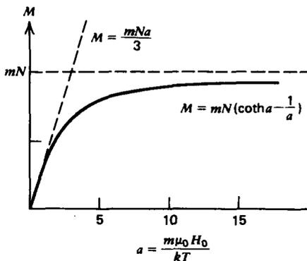
Figure 5-19 The Langevin equation describes the net magnetization. At low temperatures (high  $a$ ) all the dipoles align with the field causing saturation. At high temperatures ( $a \ll 1$ ) the magnetization increases linearly with field.
