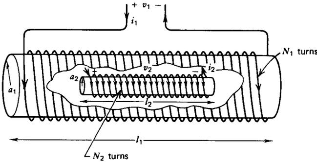
(a) Neglecting fringing field effects find the self-inductances and mutual inductances of each coil. (Hint: Assume the magnetic field is essentially uniform within the cylinders.)
