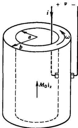
(a) If the cylinder is assumed very long compared to its radius, what are the approximate values of  $\mathbf{B}$  and  $\mathbf{H}$  in the magnet?
