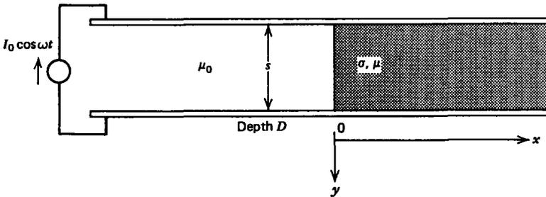
(a) What are the magnetic field and current distributions within the conducting block?
