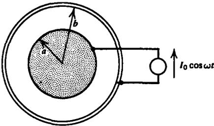
(a) Assuming that  $\mathbf{H} = H_\phi(r)\mathbf{i}_\phi$ , what is the governing equation for  $H_\phi(r)$  within the inner cylinder. (Hint:  $\nabla^2 \mathbf{H} = \nabla(\nabla \cdot \mathbf{H}) - \nabla \times (\nabla \times \mathbf{H})$ .)
