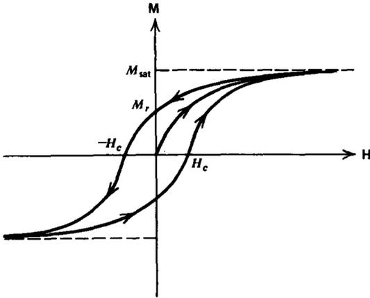
Figure 5-20 Ferromagnetic materials exhibit hysteresis where the magnetization saturates at high field strengths and retains a net remanent magnetization  $M_r$ , even when  $H$  is zero. A coercive field  $-H_c$  is required to bring the magnetization back to zero.
