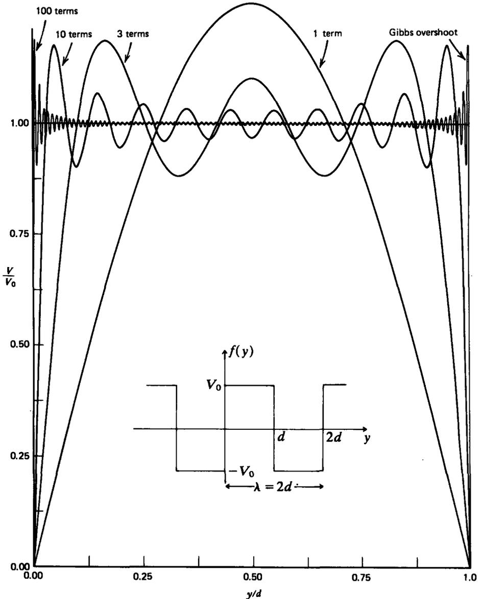
Figure 4-6 Fourier series expansion of the imposed constant potential along the  $x = 0$  edge in Figure 4-5 for various partial sums. As the number of terms increases, the series approaches a constant except at the boundaries where the discontinuity in potential gives rise to the Gibbs phenomenon of an 18% overshoot with narrow width.
