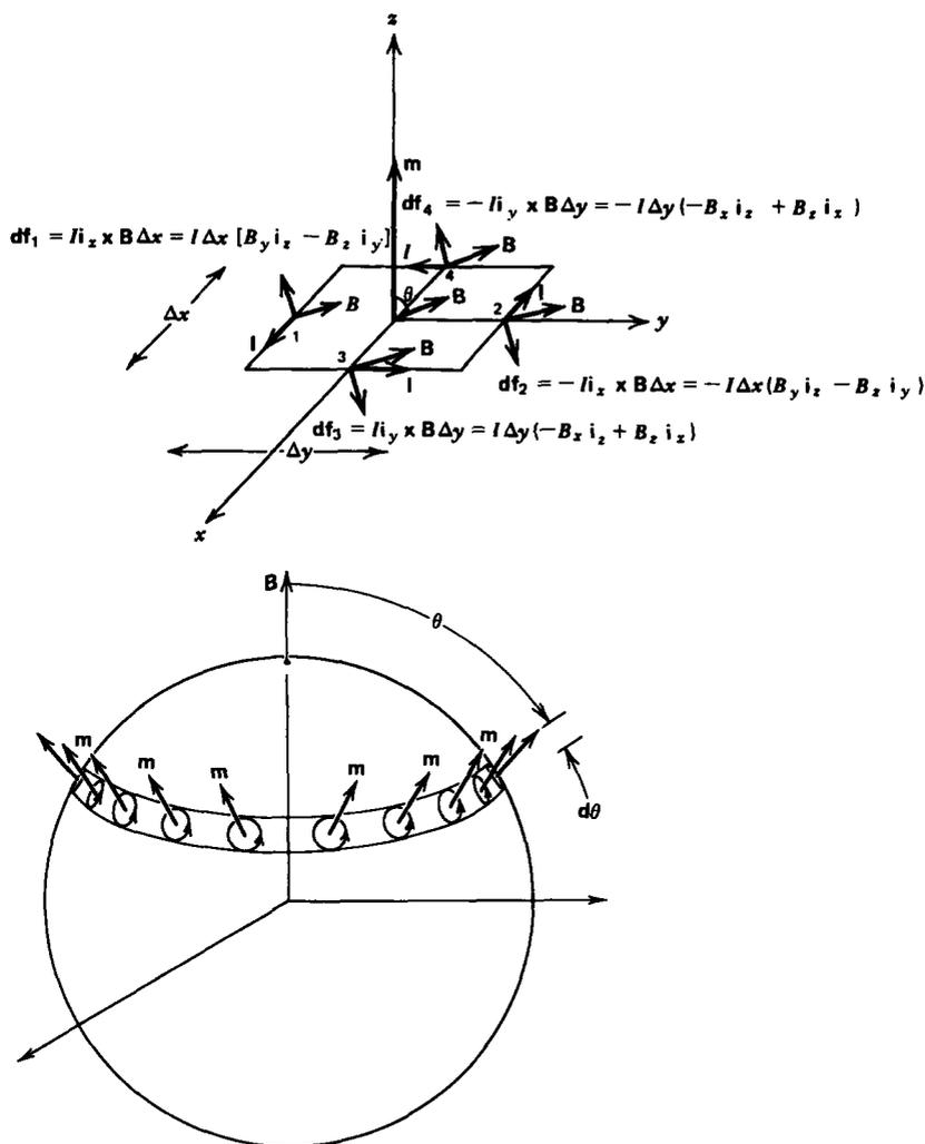
Figure 5-18 (a) A torque is exerted on a magnetic dipole with moment  $\mathbf{m}$  at an angle  $\theta$  to an applied magnetic field. (b) From Boltzmann statistics, thermal agitation opposes the alignment of magnetic dipoles. All the dipoles at an angle  $\theta$ , together have a net magnetization in the direction of the applied field.
