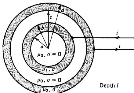
31. Find the external self-inductance of the two wire lines shown. (**Hint:** See Section 2-6-4c.)
