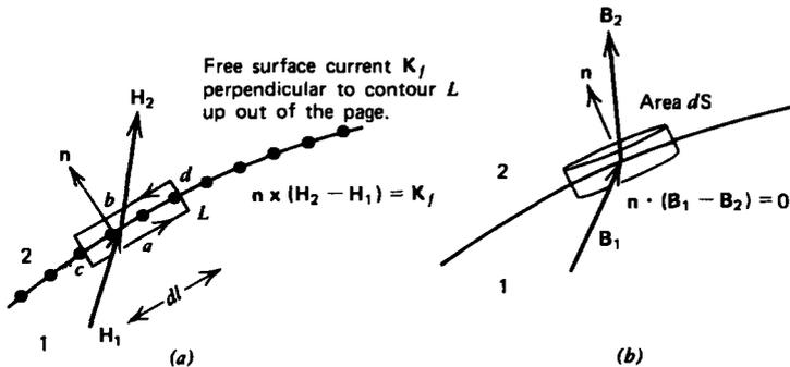
Figure 5-22 (a) The tangential component of  $\mathbf{H}$  can be discontinuous in a free surface current across a boundary. (b) The normal component of  $\mathbf{B}$  is always continuous across an interface.
