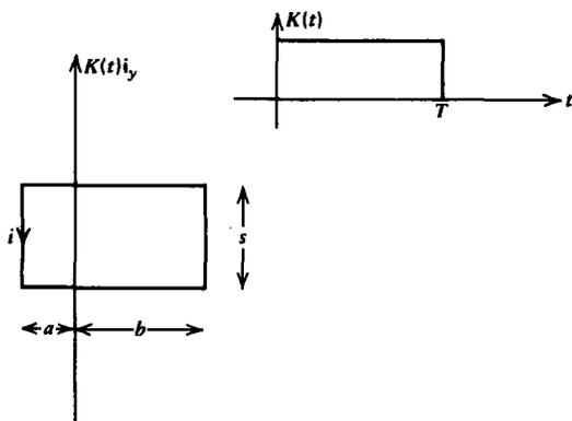
(a) The current sheet is instantaneously turned on to a dc level  $K_0\mathbf{i}_y$  at  $t=0$ . What is the induced loop current?
