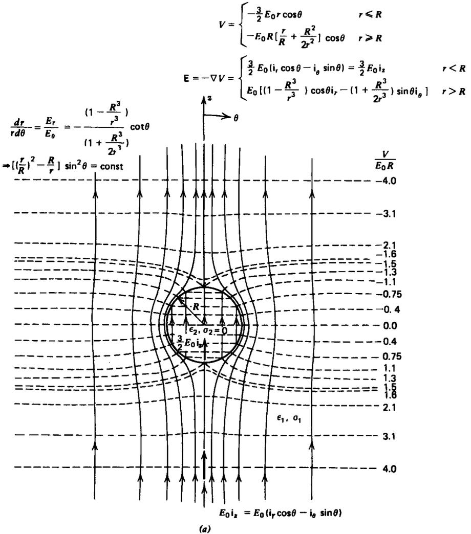
Figure 4-12 Steady-state field and equipotential lines about a (a) perfectly insulating or (b) perfectly conducting sphere in a uniform electric field.
