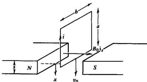
(a) What is the imposed flux through the loop as a function of the loop's position  $x$  ( $0 < x < s$ ) within the magnet?
