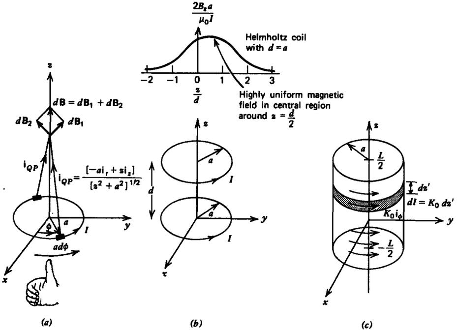
Figure 5-10 (a) The magnetic field due to a circular current loop is  $z$  directed along the axis of the hoop. (b) A Helmholtz coil, formed by two such hoops at a distance apart  $d$  equal to their radius, has an essentially uniform field near the center at  $z = d/2$ . (c) The magnetic field on the axis of a cylinder with a  $\phi$ -directed surface current is found by integrating the fields due to incremental current loops.
