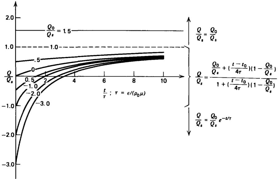
Figure 4-14 There are three regimes describing the charge build-up on the sphere. It takes many time constants  $[\tau = \epsilon/(\rho_0\mu)]$  for the charge to approach the saturation value  $Q_s$ , because as the sphere charges up the Coulombic repulsive force increases so that most of the charge goes around the sphere. If the sphere is externally charged to a value in excess of the saturation charge, it remains constant as all additional charge is completely repelled.
