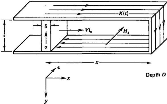
(a) The surface current on the plates  $K(t)$  will vary with time. What is the magnetic field in terms of  $K(t)$ ? Neglect fringing effects.
