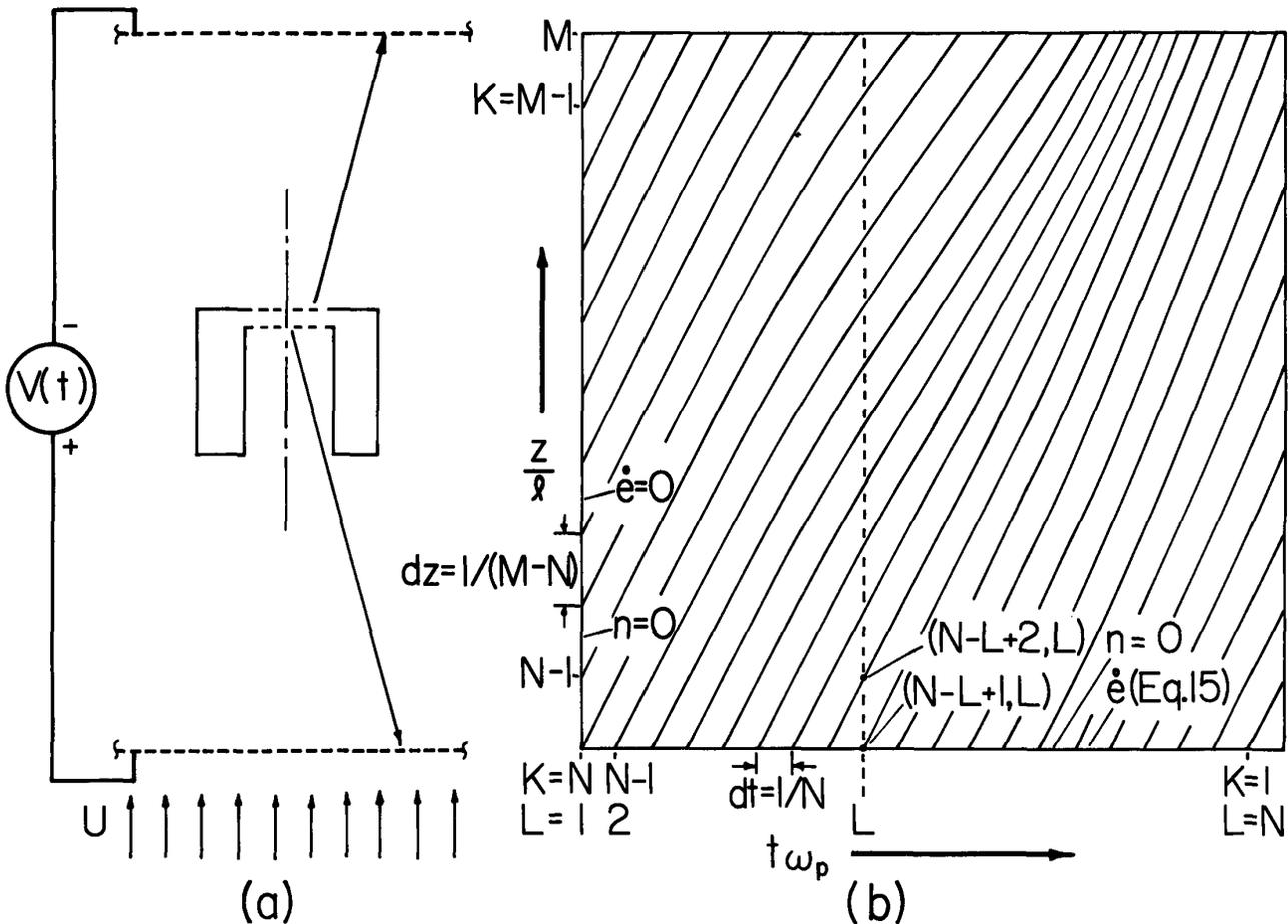
Fig. 11.9.1. (a) Beam enters region between screen electrodes with velocity  $U$ . At microwave frequencies, the screens typically provide coupling to cavity resonators, as shown by the inset. (b) Characteristic lines in the  $z$ - $t$  plane. Coordinate  $(x, t)$  is denoted by characteristic line  $(K)$  and time  $(L)$ .
