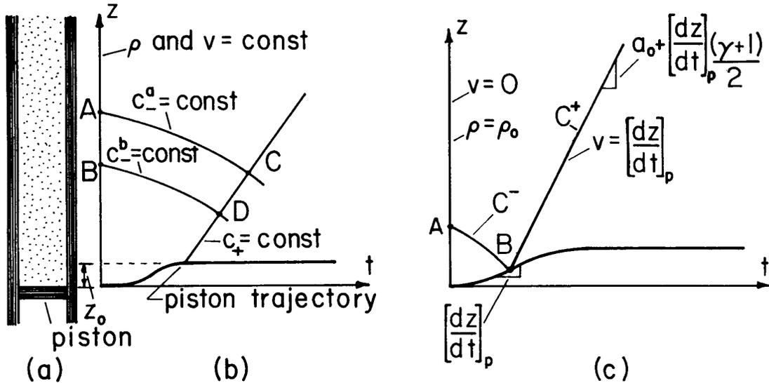
Fig. 11.7.3. (a) Gas filled tube driven by piston. (b) Boundary and initial value problem where the initial state of the fluid is uniform (when  $t = 0$ ) and an excitation is applied by means of a piston which is initially at  $z = 0$ . (c)  $a$  and  $v$  are constant along  $C^+$  characteristics, which are straight lines.
