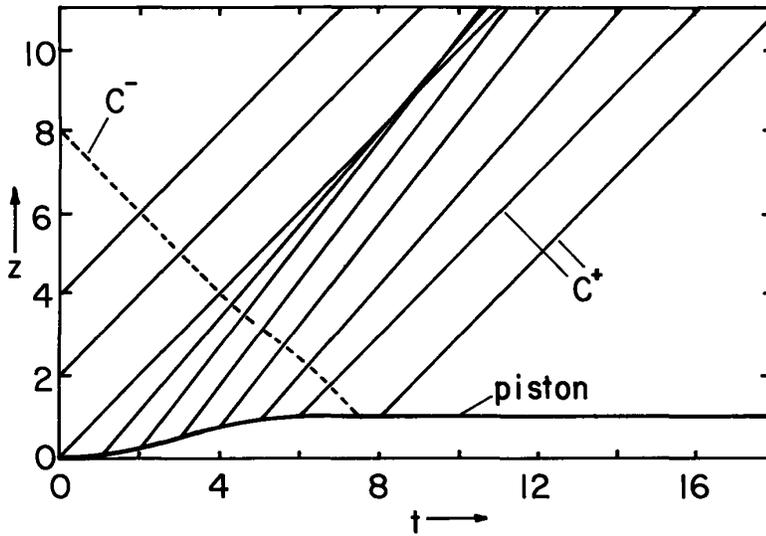
Fig. 11.7.4. Simple-wave characteristic lines initiated by piston.
