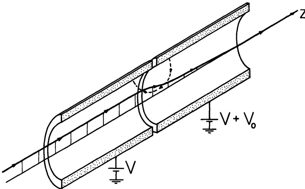
Fig. 11.4.1. (b) Electric electron beam lens with trajectory exemplified by Fig. 11.4.3.
