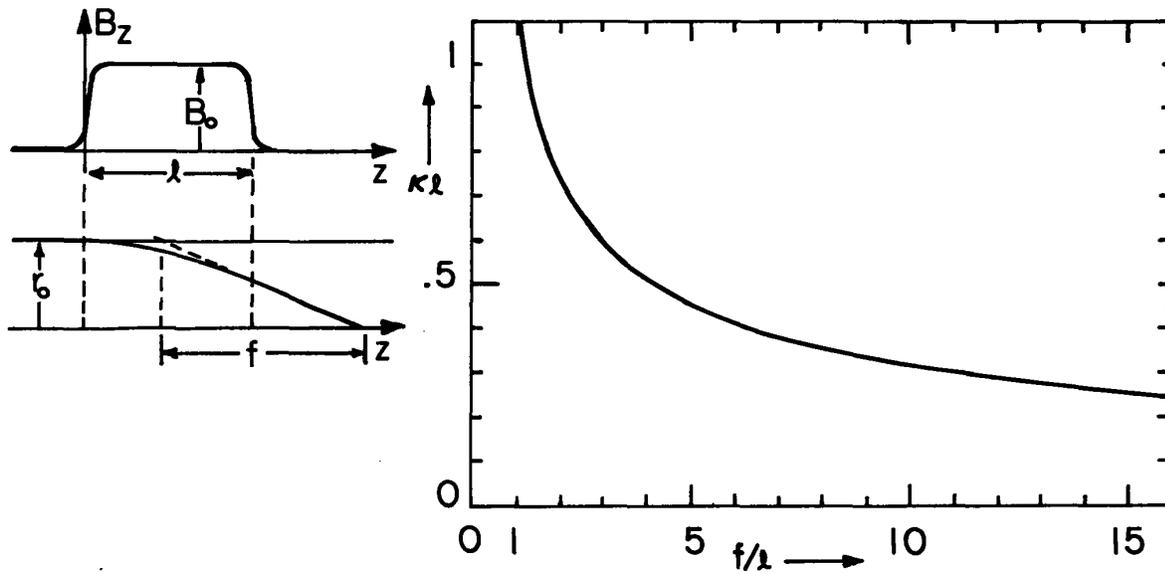
Fig. 11.4.2. For magnetic lens of Fig. 11.4.1a, having essentially uniform axial field  $B_0$  over length  $l$ , focal length  $f$  normalized to  $l$  is given as a function of  $\kappa l$ , defined with Eq. 10.
