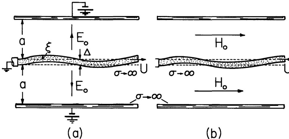
Fig. 11.10.1. Prototype single-stream systems consisting of perfectly conducting sheets convecting to the right with velocity  $U$ . (a) Potential constrained EQS configuration; (b) flux constrained MQS configuration.
