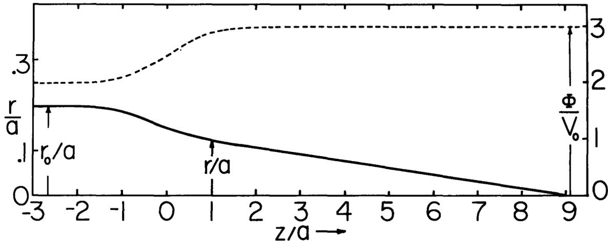
Fig. 11.4.3. For the electric lens of Fig. 11.4.1b, the axial potential distribution is represented by the broken curve. The solid curve is the electron trajectory predicted by Eqs. 13 and 14 with  $V_0/V = 0.5$  and  $\beta = 2$ .
