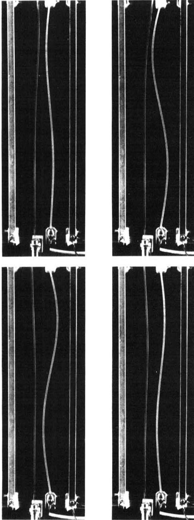
Fig. 11.16.6. Instantaneous photographs of the streaming over stability in Fig. 11.16.5. The time interval between exposures is equivalent to about  $60^\circ$  in phase. The frequency of oscillation is about 7 Hz (from film Reference 11, Appendix C).
