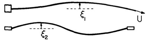
Fig. 11.16.1. Schematic of stream-structure interaction, showing three upstream boundary conditions and one downstream condition for  $M_1 > 1$  and  $M_2 = 0$ .
