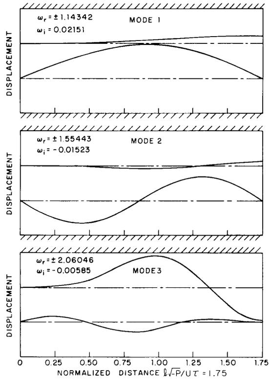
Fig. 11.16.4. Eigenfunctions for the three lowest modes for the magnetic system of Fig. 11.16.3.
