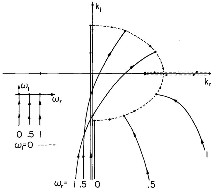
Fig. 11.12.8. Loci of  $k$  for loci of  $\omega$  shown by inset. Broken curves are values of  $k$  for real  $\omega$ . Superelectric case ( $|M| > 1$ ,  $P > 0$ ) displays amplifying waves ( $P = 1$ ,  $M = 1.5$ ).
