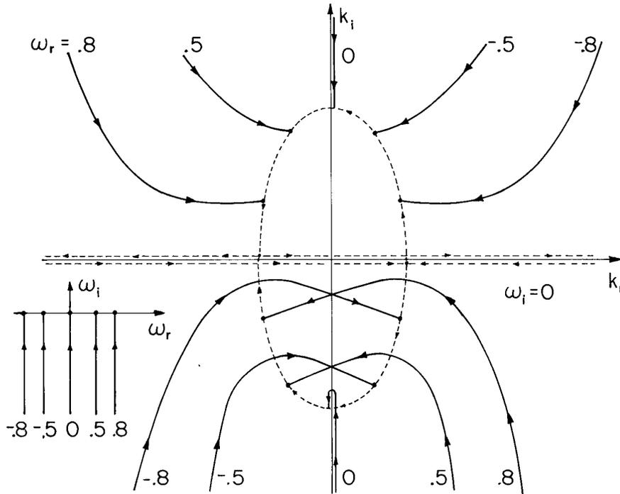
Fig. 11.12.7. Loci of  $k$  for loci of  $\omega$  shown by inset. Broken curves are values of  $k$  for real  $\omega$ . Submagnetic case ( $|M| < 1$ ,  $P < 0$ ) displays evanescent waves ( $P = 1$ ,  $M = 0.5$ ).
