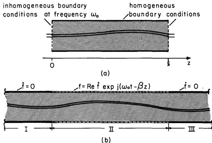
Fig. 11.11.2. Typical systems that are uniform in the  $z$  direction; (a) bounded longitudinally by planes where boundary conditions are imposed; (b) unbounded in the  $z$  direction with drive from a transverse boundary over the interval  $0 < z < \ell$ .
