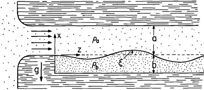
In stationary state, lower fluid is static while upper one streams to the right with uniform velocity  $U$ . At the interface there is a discontinuity in fluid velocity, and hence a vorticity sheet.
