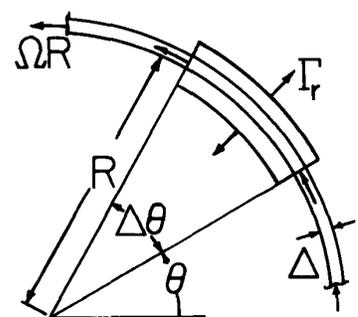
Fig. 10.5.2. Incremental section of thermally conducting moving shell.
