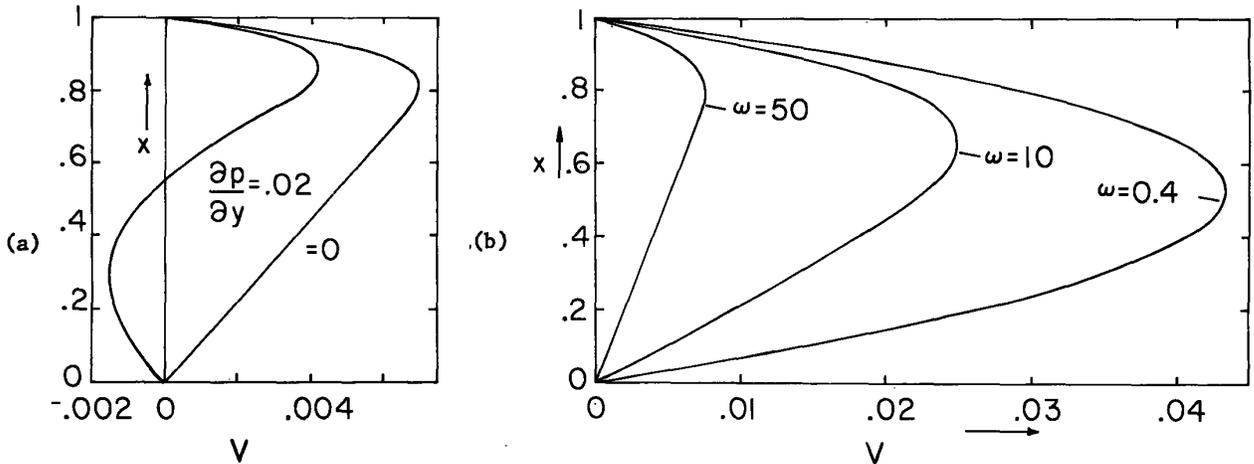
Fig. 9.5.2. (a) Normalized velocity profile with pressure gradient as parameter.  $\omega = 50$  ( $\delta'/a = 0.2$ ) and  $k = 1$ . (b) Normalized velocity profile with zero pressure gradient showing effect of frequency  $\omega$ . For  $\omega = 50$ , the force density is confined to upper 20% of layer so that profile in the region below is the linear one typical of Couette flow.
