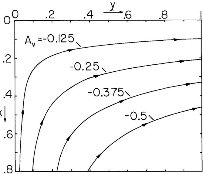
Fig. 9.7.9. Streamlines for stress-constrained boundary layer, as would result in configuration of Fig. 9.7.6. Variables are normalized.
