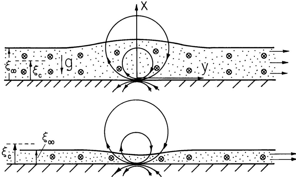
Fig. 9.14.3. Conservative transition of steady flow carrying uniform current density in  $z$  direction as it passes through field of magnetic dipole: (a) subcritical entrance; (b) supercritical entrance.
