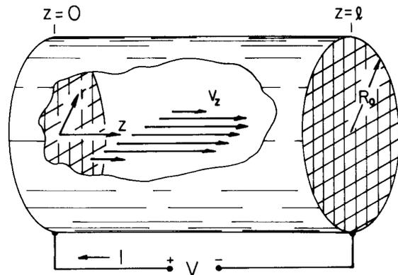
Fig. 9.12.1. Circular cylindrical conduit having insulating wall supporting screens at  $z = 0$  and  $z = \ell$ . Charged particles are injected at left and pulled through the fluid to provide electrohydrodynamic pumping. Flow is electric analogue of Hartmann flow.
