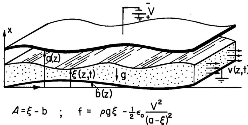
Fig. 9.13.1. Gravity flow with constant potential interface stressed by electric field. Quasi-one-dimensional model expressed by Eqs. 11 and 12 reduces to classic gravity-wave model if  $V = 0$ . The hydromagnetic flux conserving antidual of this potential conserving continuum is suggested by Sec. 8.5.
