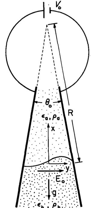
Fig. 8.11.1. Cross section of experiment shown in Fig. 8.9.3a with Cartesian coordinates for planar model.
