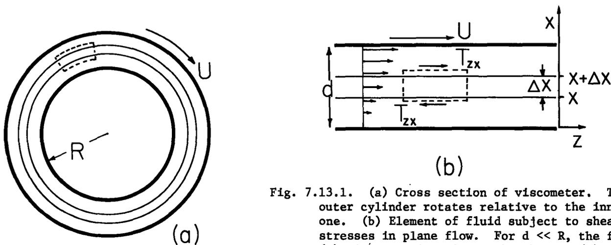
Fig. 7.13.1. (a) Cross section of viscometer. The outer cylinder rotates relative to the inner one. (b) Element of fluid subject to shear stresses in plane flow. For  $d \ll R$ , the flow, (a), is approximately as sketched in (b).
