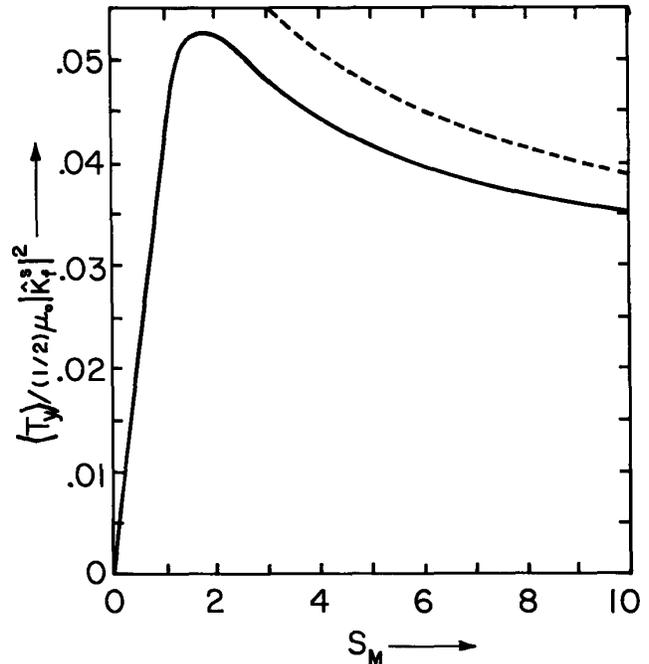
Fig. 6.6.2. Time-average force/unit area acting on deep conductor in direction of traveling wave.  $ka=kd=1$ ,  $\mu=\mu_0$ . The force is an odd function of  $S_M \equiv \mu\sigma a^2(\omega - kU)$ . The broken curve is the high-frequency asymptote given by Eq. 11.
