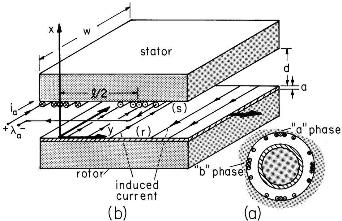
Fig. 6.4.1. (a) Cross section of rotating induction machine with thin-sheet conductor on rotor. (b) Developed model for (a) with air gap  $d$  and sheet conductor of thickness  $a$ . One of two phases on the stator is shown.
