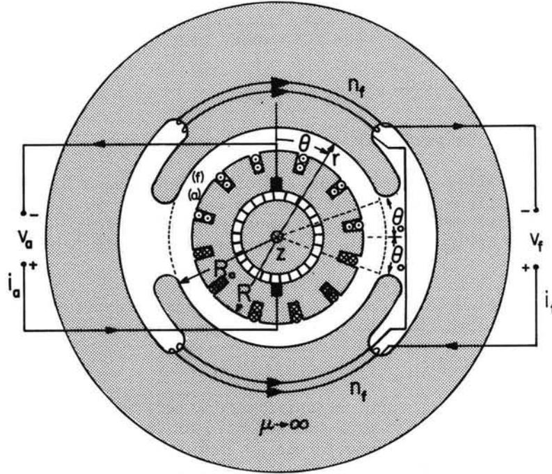
Fig. 4.10.1. Cross section of d-c machine.
