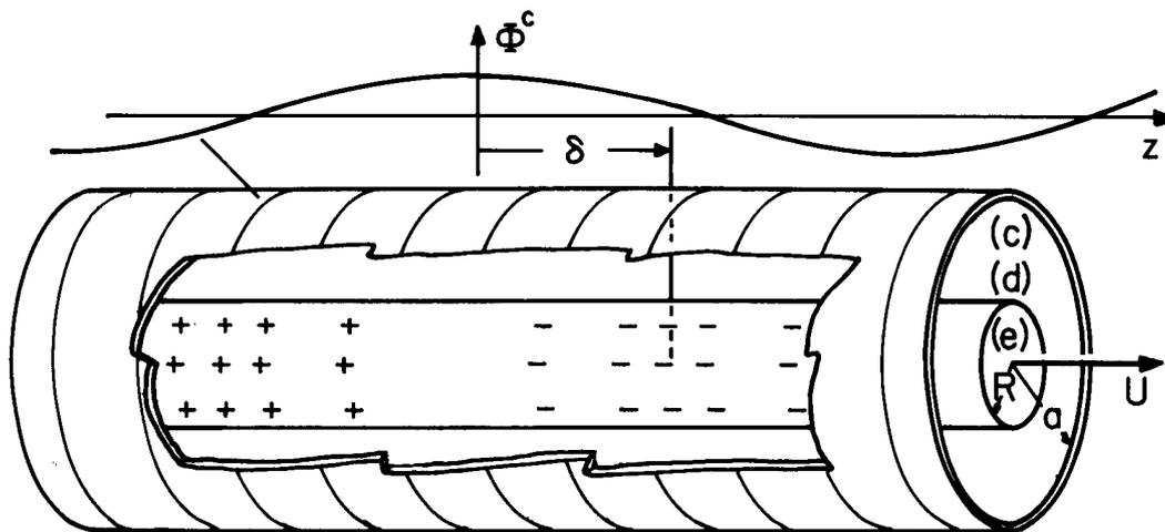
Fig. 4.6.1. Regions of positive and negative charge represent concentrations and rarefactions in the local charge density of an initially uniformly charged beam moving in the  $z$  direction with the velocity  $U$ .
