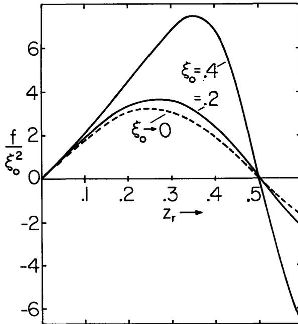
Fig. 4.13.2a. Electrical force on rotor of variable-capacitance machine (Fig. 4.12.1) as a function of normalized relative displacement  $z_r = z_r/\lambda$ , with amplitude of electrodes as a parameter.
