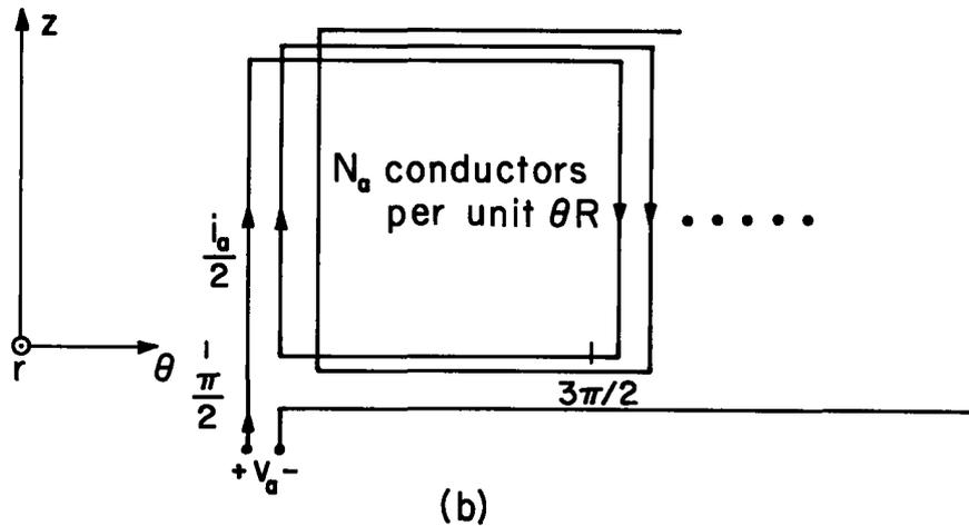
Fig. 4.10.3. (a) Typical winding scheme for armature of d-c machine shown in Fig. 4.10.1. The  $r$  axis is directed out of the paper. Brushes make contact with commutator segments which move to the right with armature conductors.<sup>2</sup> (b) Winding distribution of solid wires.
