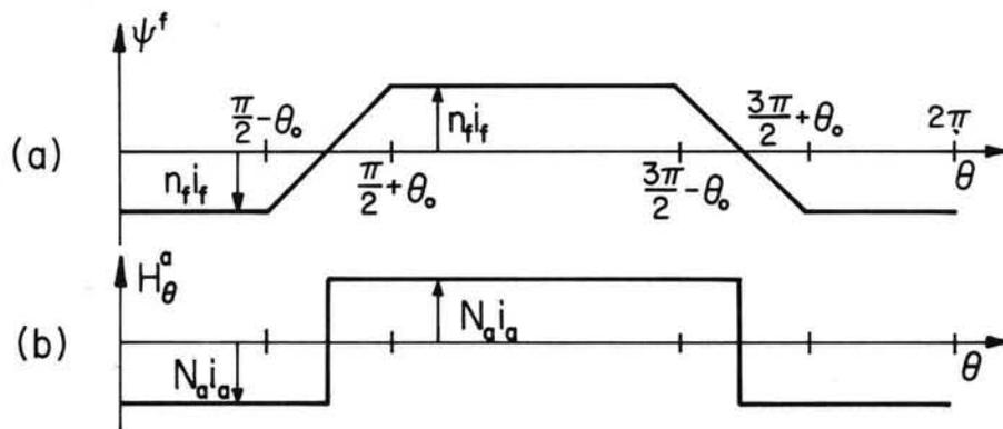
Fig. 4.10.2. Circumferential distribution of magnetic potential at  $r = R_0$  and tangential magnetic field intensity at  $r = R$ .
