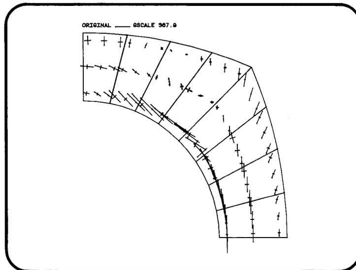
Finite element mesh to be generated using ADINA-IN:
