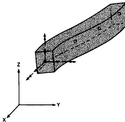
Isoparametric Beam Element
