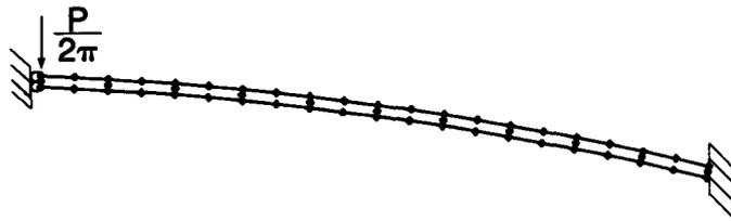
Deformed configuration for  $P = 100 \text{ lb}$ :
