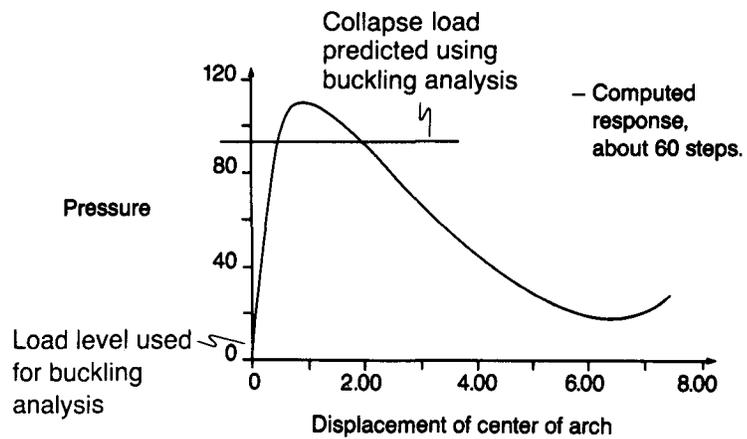
We have computed the response of a perfect (symmetric) arch. Because the first collapse mode is antisymmetric, that mode is not excited by the pressure loading during the response calculations.
