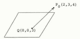
Thus, the distance from  $P_0$  to the plane is the length of the projection of  $P_0^{\dagger}Q$  in the direction of the normal to the plane and this in turn is given by  $|P_0^{\dagger}Q \cdot u_N|$ , where  $u_N^{\dagger}$  is a unit normal to the plane. Since the equation of the plane is 4x + 5y + 2z = 6, a normal to the plane is 4i + 5j + 2k. Hence, a unit normal is
