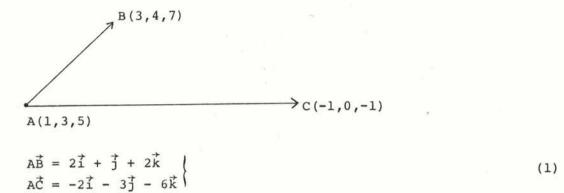
Now  $\overrightarrow{AB} + \overrightarrow{AC}$  is the vector which is the <u>diagonal</u> of the parallelogram determined by A, B, and C. In general, such a diagonal <u>does not</u> bisect the vertex angle. In fact it bisects the angle if and only if the parallelogram is a rhombus (all four sides have equal length).
