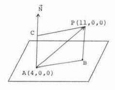
Notice our orientation. Certainly (11,0,0) and (4,0,0) should lie on the x-axis. That is AP is a segment of the x-axis. The point is that PB does not represent the direction of the z-axis in our diagram.
