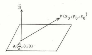
Equation of plane is ax + by + cz = d. Therefore, we may let  $A(\frac{d}{a},0,0)$  denote a point in the plane (if a = 0 we work with  $(0,\frac{d}{b},0)$ , etc.).
