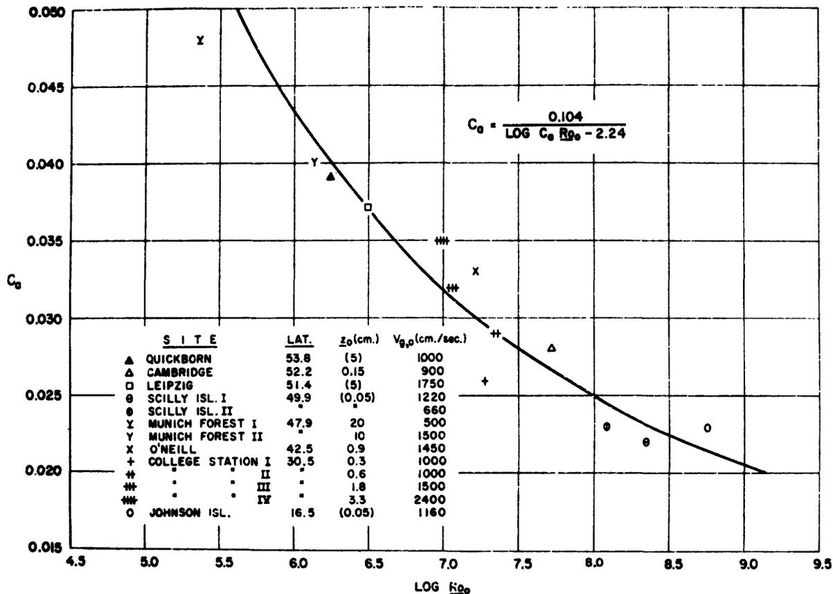
Figure 17.16 Geostrophic drag coefficient versus surface Rossby number.  $C_g = u_*/|V_g|$ ,  $R_{g0} = |V_g|/(fz_0)$ . (Lettau, 1959.)
