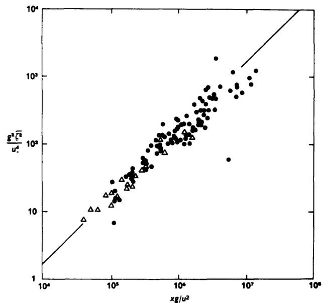
Figure 17.4 Field measurements of the dimensionless mean-square displacement  $g^2 \zeta^2 / u_*^4$  as a function of dimensionless fetch  $Xg / u_*^2$ . Data points are represented thus: Hasselmann et al. (1973),  $\bullet$ ; Burling (1959),  $\Delta$ . The line in the background is  $g^2 \zeta^2 / u_*^4 = 1.6 \times 10^{-4} Xg / u_*^2$ . (Phillips, 1977a.)
