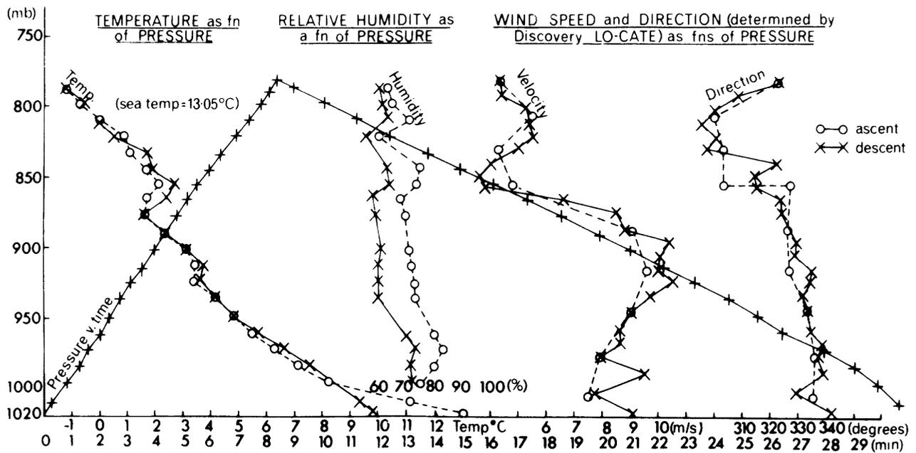
Figure 17.11 Records from LOCATE sonde (D.22) released from R.R.S. *Discovery* at 1915Z on 17 June 1970 near OWS Julliett, 52°30'N, 20°W. The record of pressure against time shows a rapid double-balloon ascent to a chosen height
