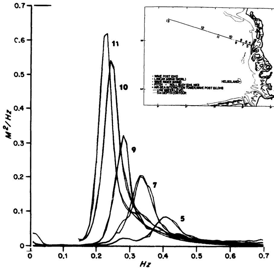
Figure 17.6 Evolution of wave spectrum with fetch for offshore winds 11<sup>h</sup>–12<sup>h</sup> Sept. 15, 1968. Numbers refer to stations inset. (Hasselmann et al., 1973.)
