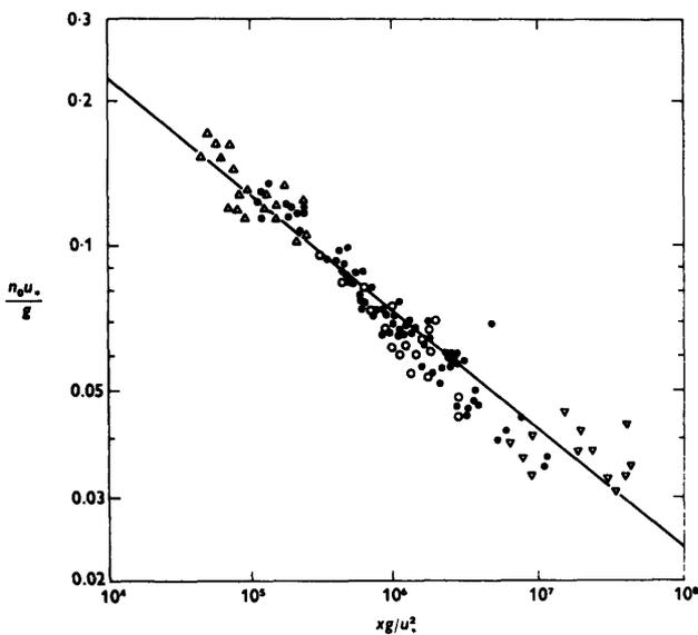
Figure 17.7 Field measurements of the dimensionless frequency of the spectral peak  $n_0 u_* / g$  vs. dimensionless fetch  $Xg/u_*^2$ . Data points are as follows: Hasselmann et al. (1973), ●; Kitaigorodskii and Strekalov (1962), ▽; Mitsuyasu (1966), ○; and Burling (1959), △. The straight line in the background is  $(n_0 u_* / g) = 2.2(Xg/u_*^2)^{-1/4}$ . [After Phillips (1977a), who compiled and plotted the original observations.]
