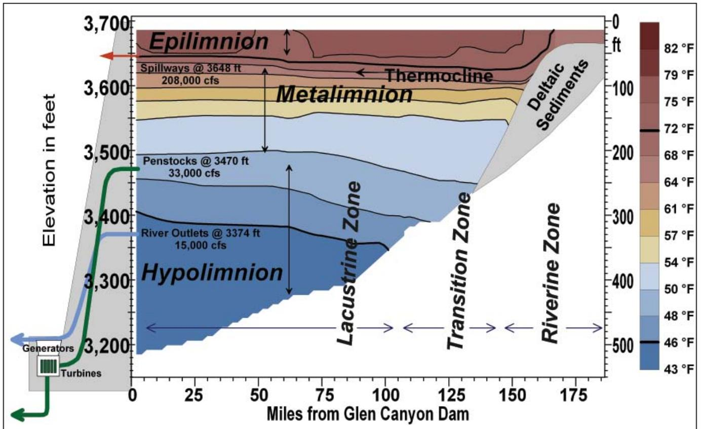
**Figure 1.** Profile of Lake Powell from Glen Canyon Dam to the inflow of the Colorado River, illustrating the vertical stratification and horizontal zonation of the reservoir at or near full pool elevation, September 1999. Also shows the elevations of each of the three release structures and their capacities as well as an approximation of the wedge of deltaic sediments. Y axis on left is measurement of elevation above mean sea level and on right is actual depth.
