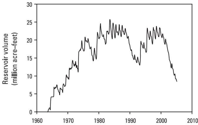
**Figure 1.** Fluctuations in the level of Lake Powell following closure of Glen Canyon Dam in 1963 (from [www.summittech.com/LakePowell/LP\\_waterDB.php](http://www.summittech.com/LakePowell/LP_waterDB.php), accessed February 20, 2005).
