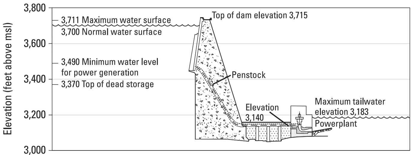
**Figure 2.** Important operating elevations of Glen Canyon Dam and Lake Powell in feet above mean sea level (msl).
