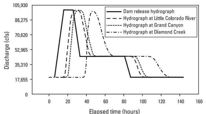
**Figure 13.** Hypothetical Glen Canyon Dam release and flow hydrographs designed to create a peak discharge of 100,000 cfs for 1 min at Diamond Creek, followed by a beach-building discharge of 45,000 cfs for a duration of 2 d.
