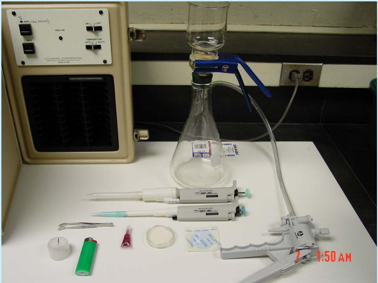
Simplified Membrane Filtration Set-up
