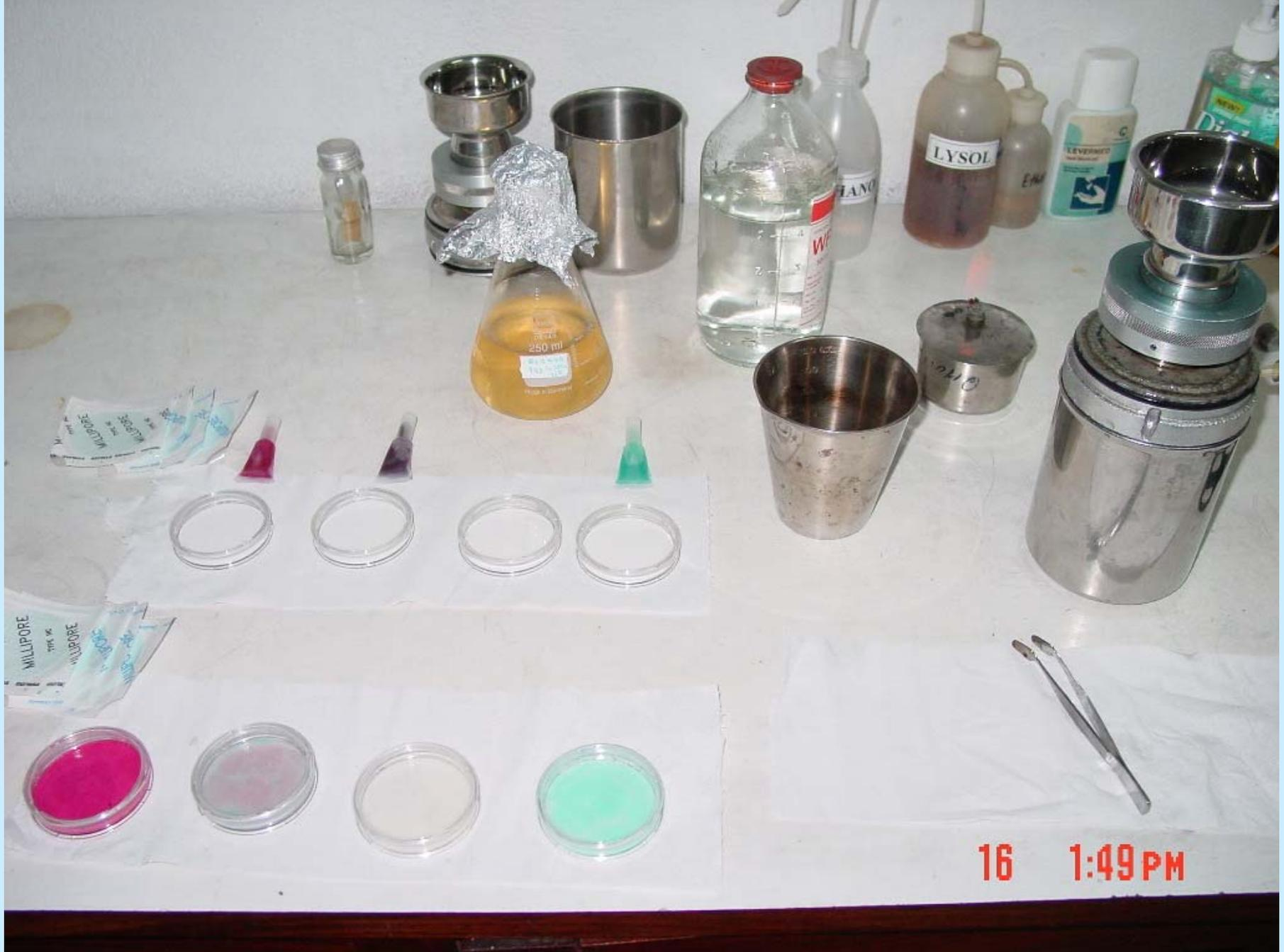
Membrane Filtration Setup with Portable Filtration Unit
