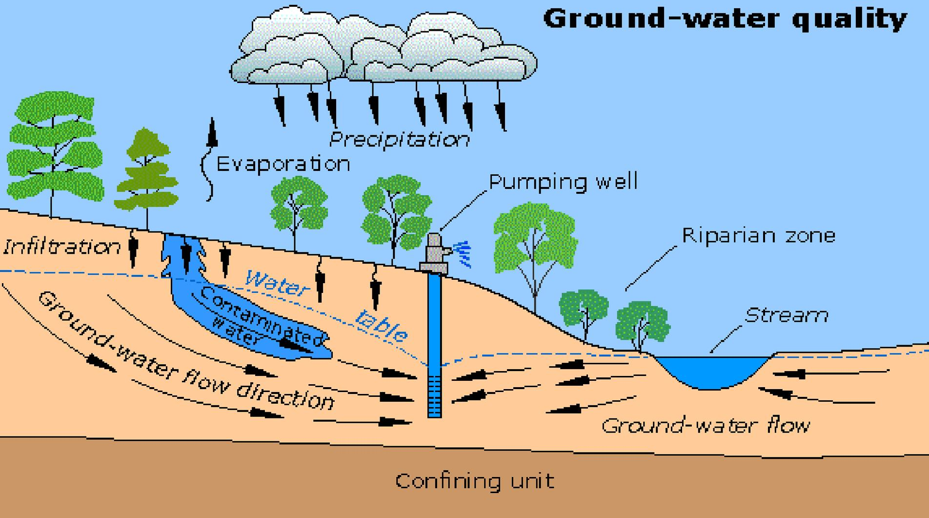
Contaminants introduced at the land surface may infiltrate to the water table and flow towards a point of discharge, either the well or the stream. (Not shown, but also important, is the potential movement of contaminants from the stream into the ground-water system, or naturally occurring toxins, such as arsenic or fluoride.)
