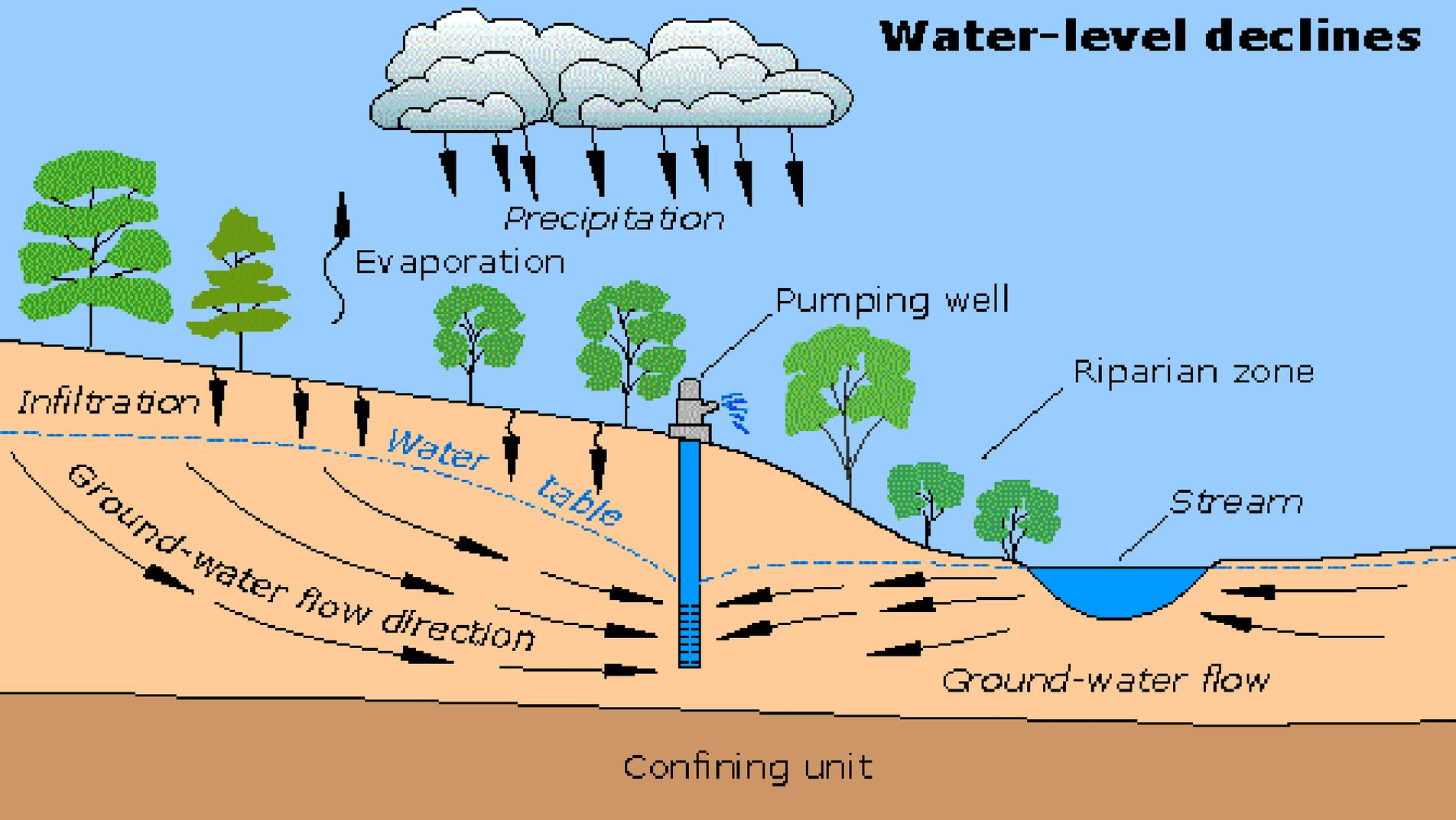
Water pumped from the ground-water system causes the water table to lower and alters the direction of ground-water movement. Some water that flowed to the stream no longer does so and some water may be drawn in from the stream into the ground-water system thereby reducing the amount of streamflow. (USGS, 2006)
