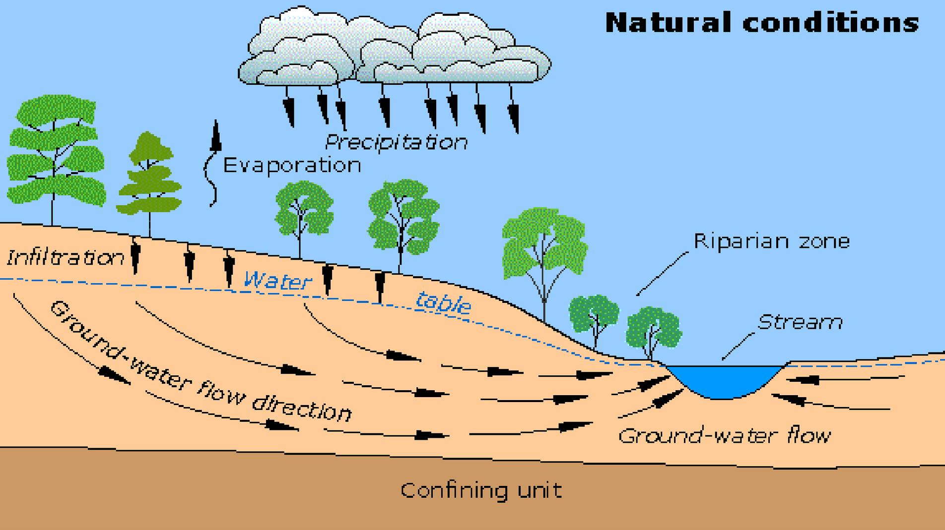
Water is recharged to the ground-water system by percolation of water from precipitation and then flows to the stream through the ground-water system. (USGS, 2006)
