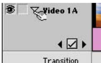
There’s now a little box with a checkmark and black arrows on either side. With the clip you put the image pan on selected, click on the left arrow. This moves the edit line to the beginning of the clip.
