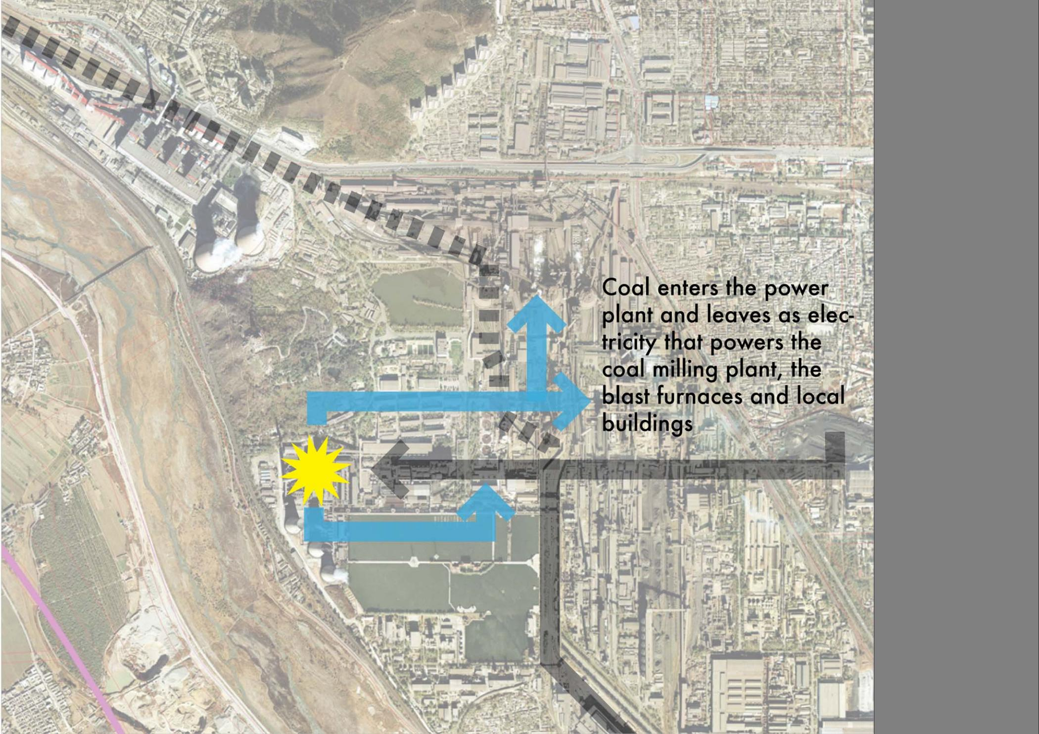
Coal enters the power plant and leaves as electricity that powers the coal milling plant, the blast furnaces and local buildings
