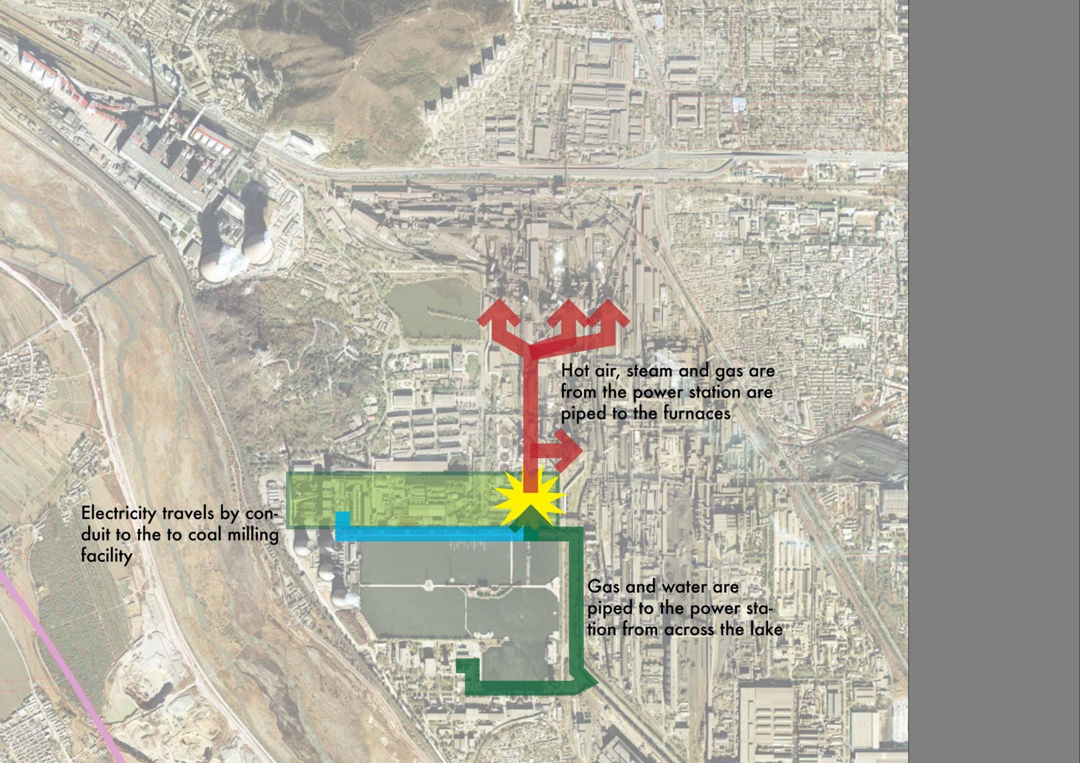
Electricity travels by conduit to the coal milling facility
