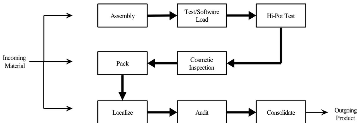
**FIGURE 1: PC FINAL ASSEMBLY PROCESS**
