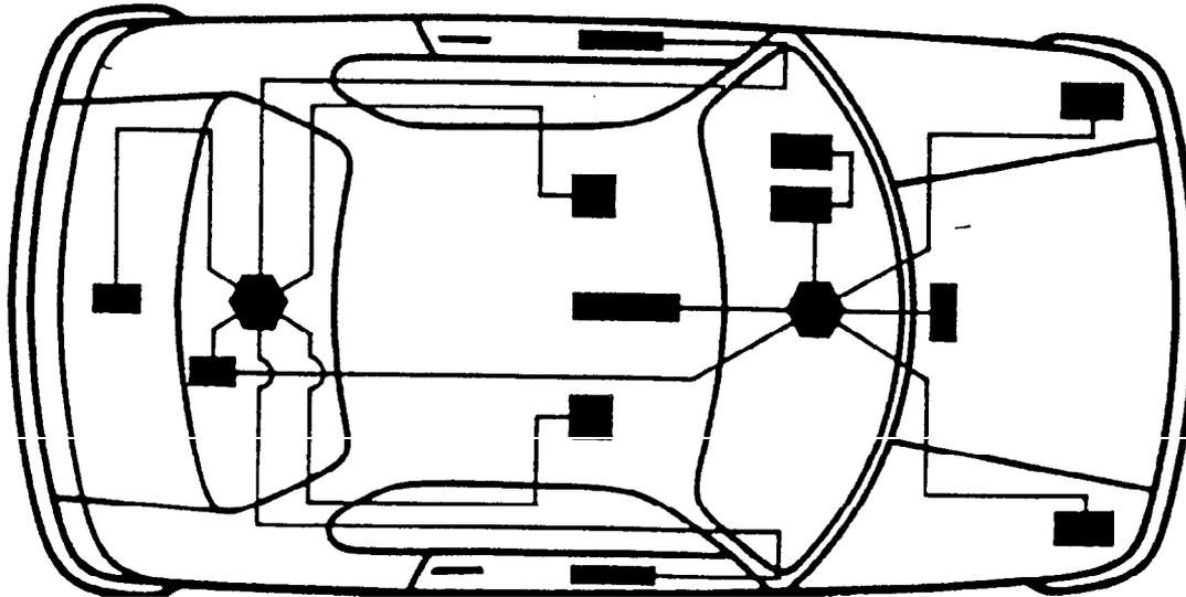
Topography of vehicle multi-plex system with central control, modules for the instrument readings, lights, doors, seats, centre console and central rear light unit.
