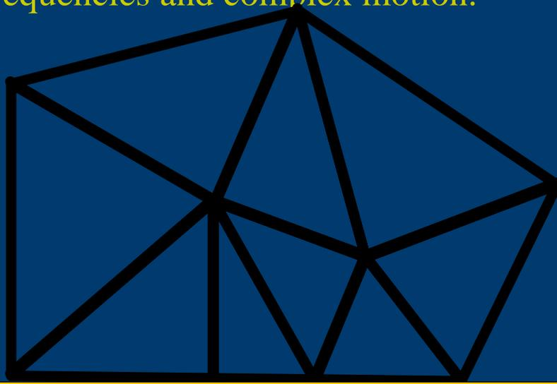
**Truss : Model as Lumped Masses with Connecting Springs**
