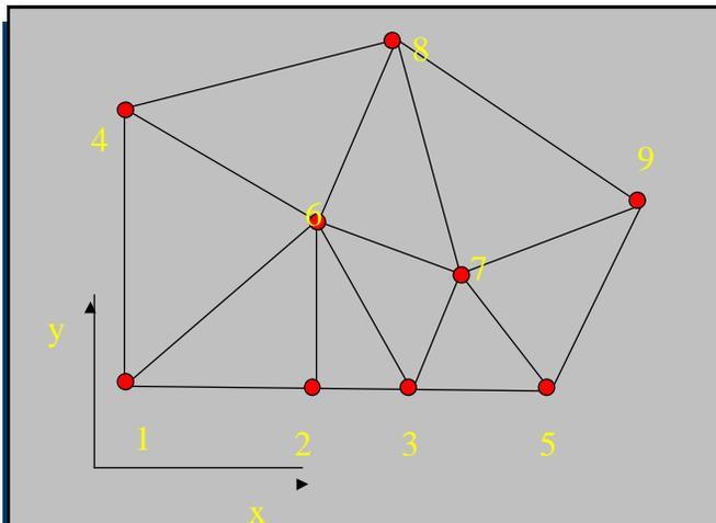
Step 6. Determine System of Equations by applying Newton's Law at each node (on each ball of mass)
