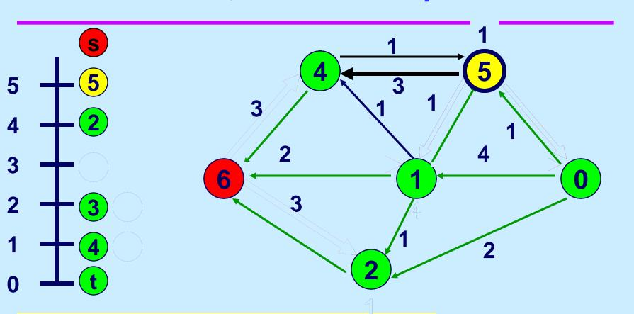
One can keep pushing flow between nodes 2 and 5 until eventually all flow returns to node s.
