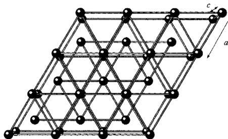
Figure 2.19. Top view of an hcp lattice.
